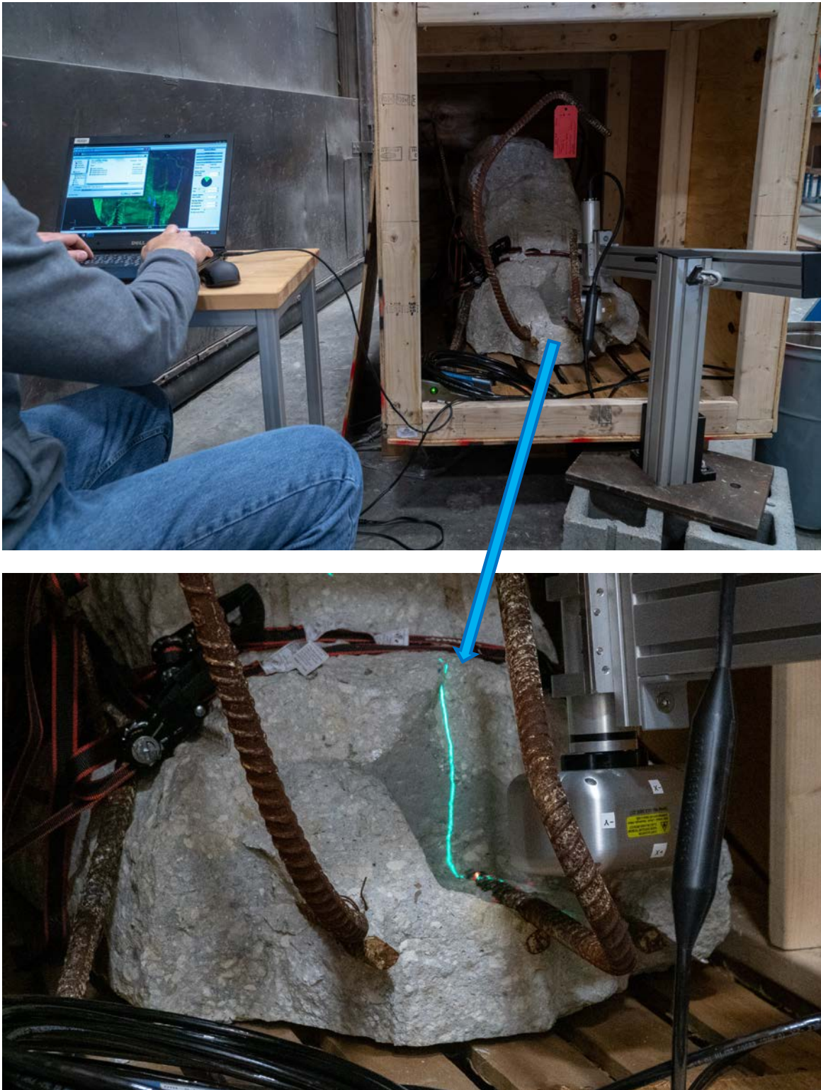
Figure 6: Macro photos of a laser scan of the flat area on the bottom of Member 12. The green line in the bottom image is the laser projected onto the surface.
