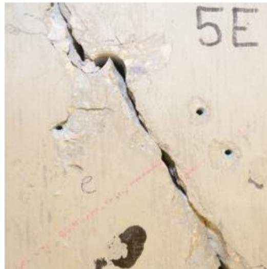
Figure 4.12. Specimen 5 after failure: overall view looking southwest (left); close-up of sliding on east side (right)
