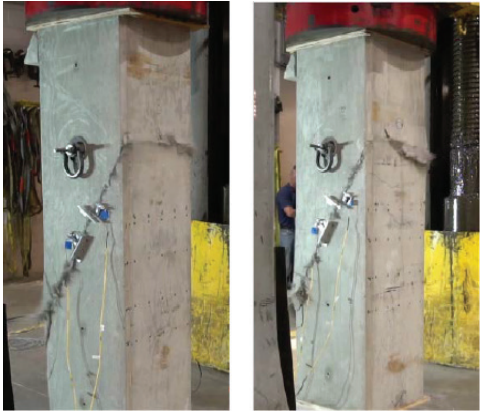
FIGURE 6-28 The moment of failure for two specimens captured from video of the tests. (Source: WJE)
