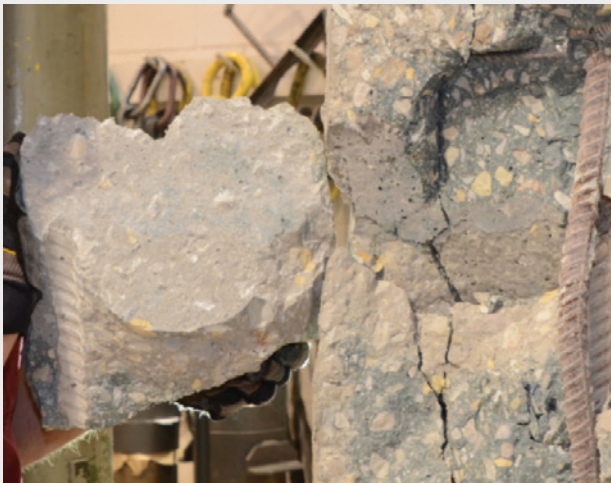
FIGURE 6-31 Construction joint interface surface after failure for an as-placed (non-roughened) specimen on the top, compared to the actual interface under member 12 on the bottom. (Source: WJE and NTSB Material Laboratory Study Report 19-043)
