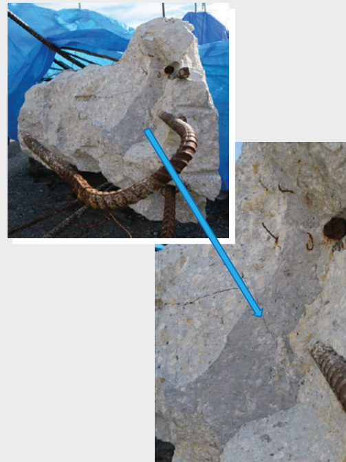
FIGURE 6-31 Construction joint interface surface after failure for an as-placed (non-roughened) specimen on the top, compared to the actual interface under member 12 on the bottom. (Source: WJE and NTSB Material Laboratory Study Report 19-043)
