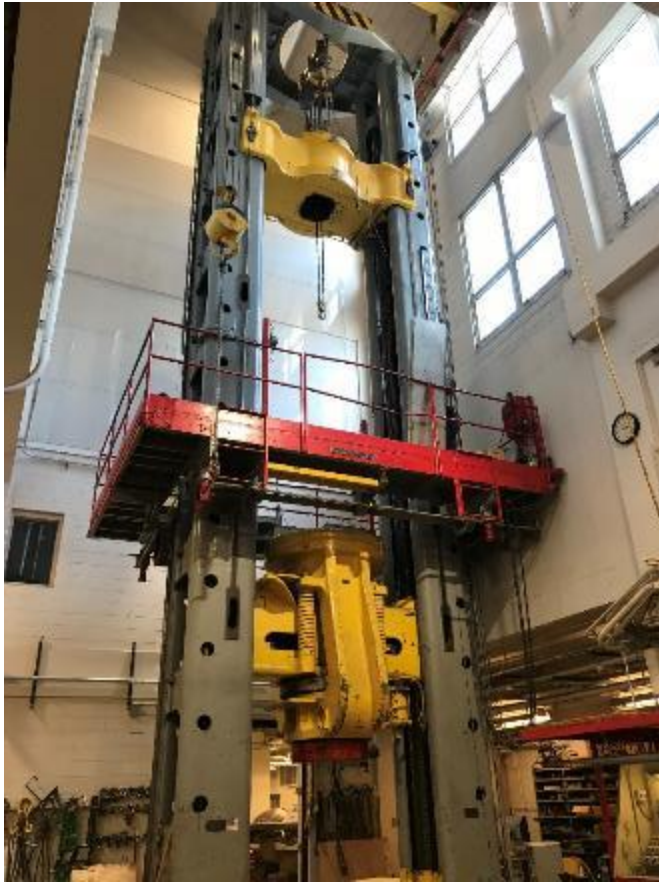
Figure 4.10. University of Illinois Southwark-Emery test machine
