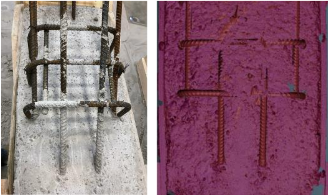
Figure 4.7. Photograph and laser scan of Specimen 3 (as-placed). (Note: the mortar adhering to the reinforcing bars in the left photo was removed before scanning and placement of the upper lift.)
