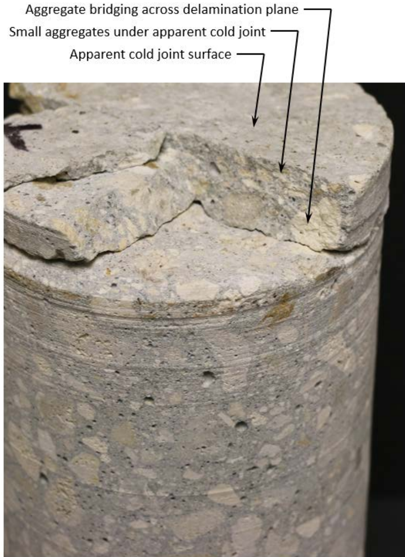
Figure 10. Annotated image of core extracted from south end of interface surface under Member 11.
