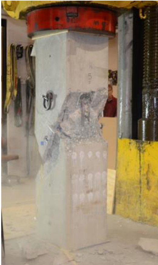
Figure 4.12. Specimen 5 after failure: overall view looking southwest (left); close-up of sliding on east side (right)
