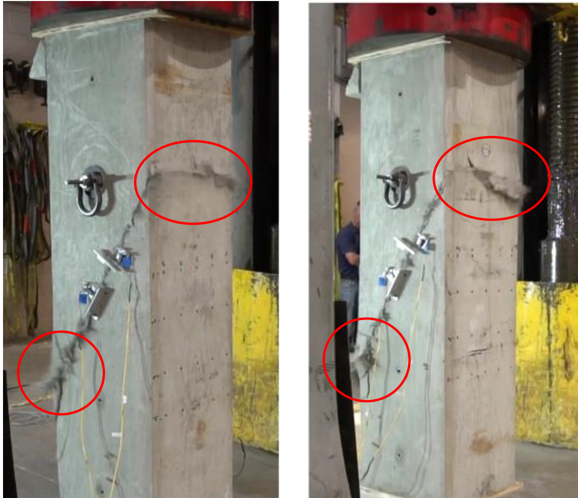
Figure 4.13. Screenshots from slow-motion video showing instant of failure: Specimen 3 (left) and Specimen 6 (right)
