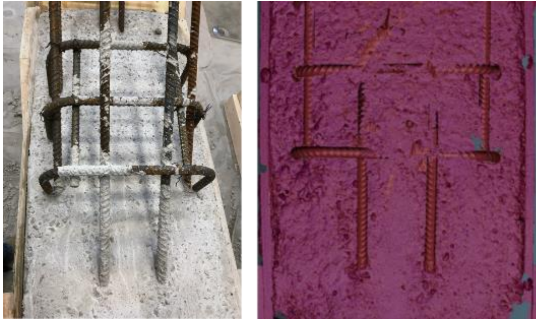
Figure 3.6. Photograph and laser scan of Specimen 3 (as-placed). (Note: the mortar adhering to the reinforcing bars in the left photo was removed before scanning and placement of the upper lift.)
