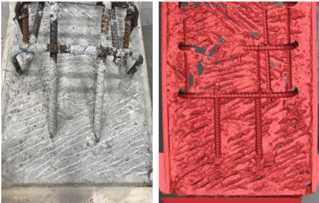
Figure 4.8. Photograph and laser scan of Specimen 4 (roughened in accordance with FDOT Standard Specifications). (Note: the mortar adhering to the reinforcing bars in the left photo was removed before scanning and placement of the upper lift.)
