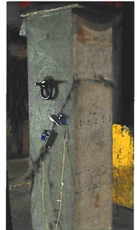
Specimen at Failure Load
