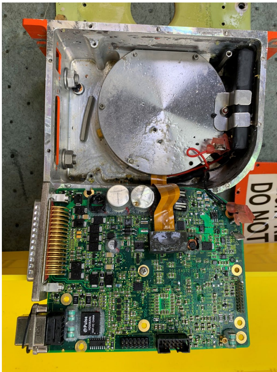
Figure 2. LDR internals exposed showing backup power supply shorted to crash-survivable case.
