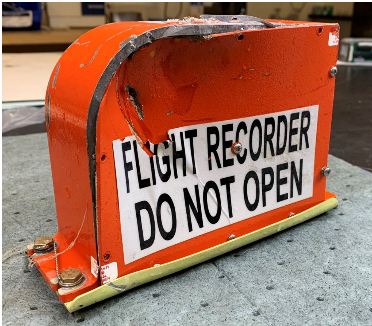
Figure 1. Condition of recorder after removal from water upon arrival at lab.
