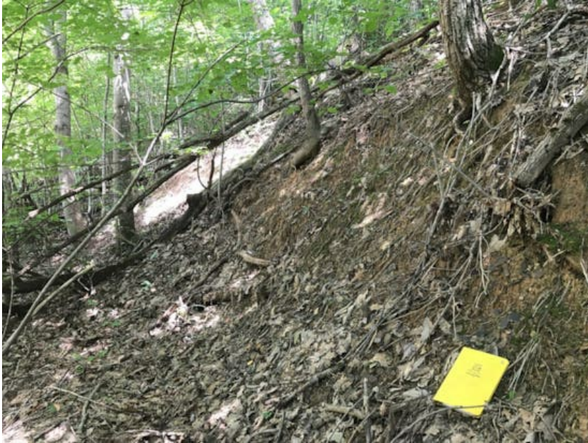
Looking north at head scarp east of ROW (Feature D). Note some fresh soil and pistol-butted trees.
