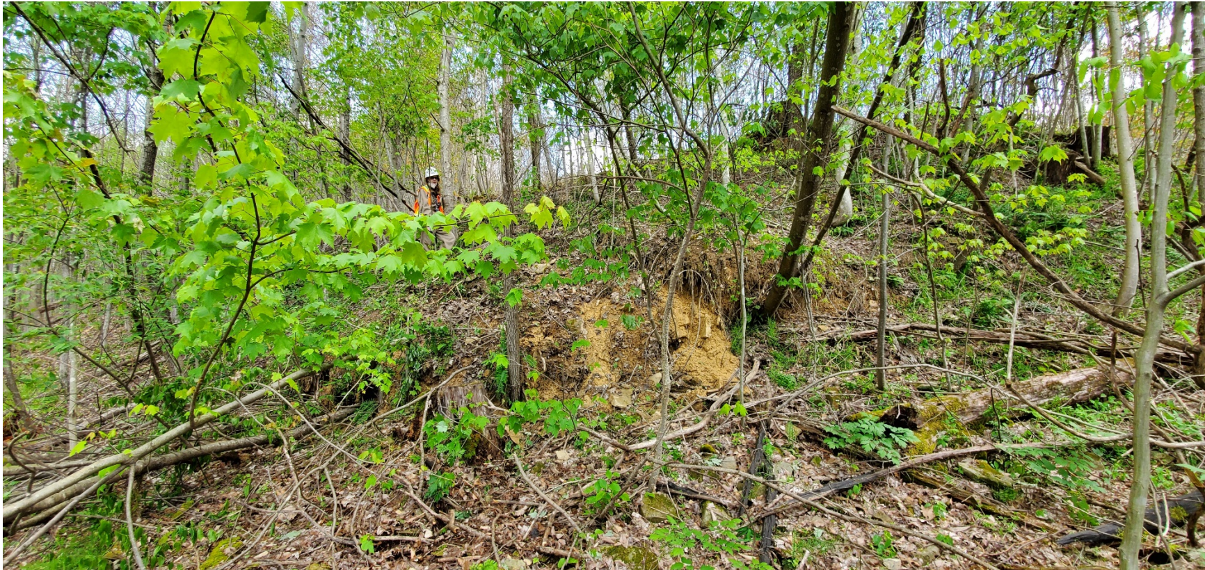
Photo C-6. Looking southeast (upslope) at the active toe. Note the fresh, saturated soil and the living trees being overridden by the landslide toe. BGC photo taken May 7, 2020.
