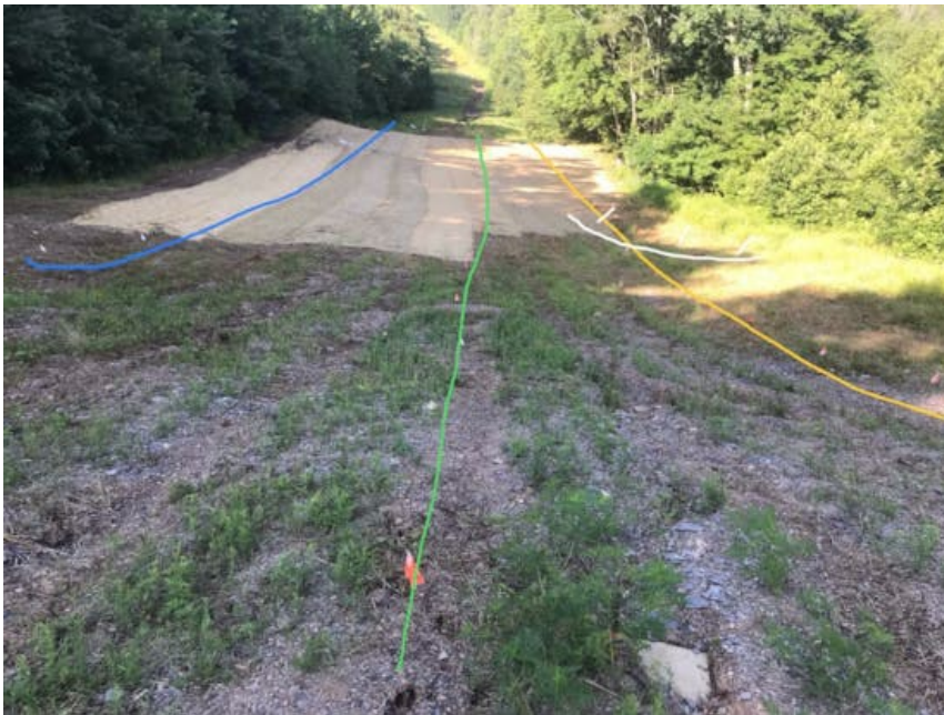
Standing on Line 15, looking downslope. Note defelction in flag lines for Line 10 (yellow) and Line 15 (green). Possible scarp noted in white. Evidence of weathered siltstone from Feature A is present in foreground.
