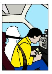
The safety belt should be placed low on your hipbones so that the belt loads will be taken by the strong skeleton of your body. If the safety belt is improperly positioned on your abdomen, it can cause internal injuries. If the safety belt is positioned on your thighs, rather
