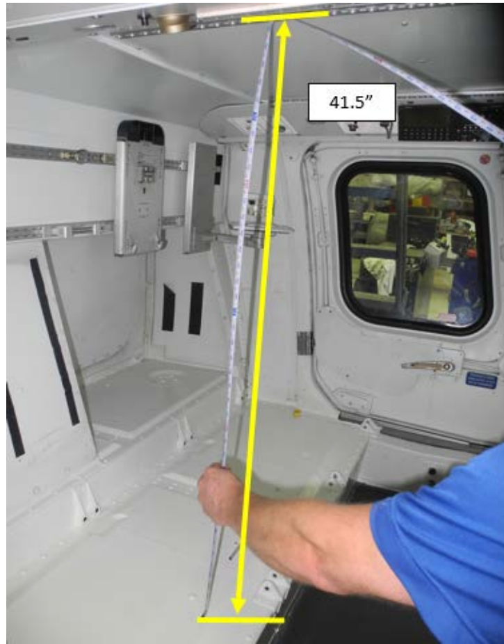
Photograph 9 - Distance From Top of Inegrated Boxed Structure to Ceiling
