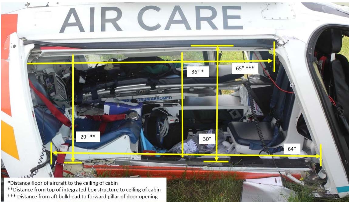
Photograph 7 – Right Side Cabin Structure Measurements
