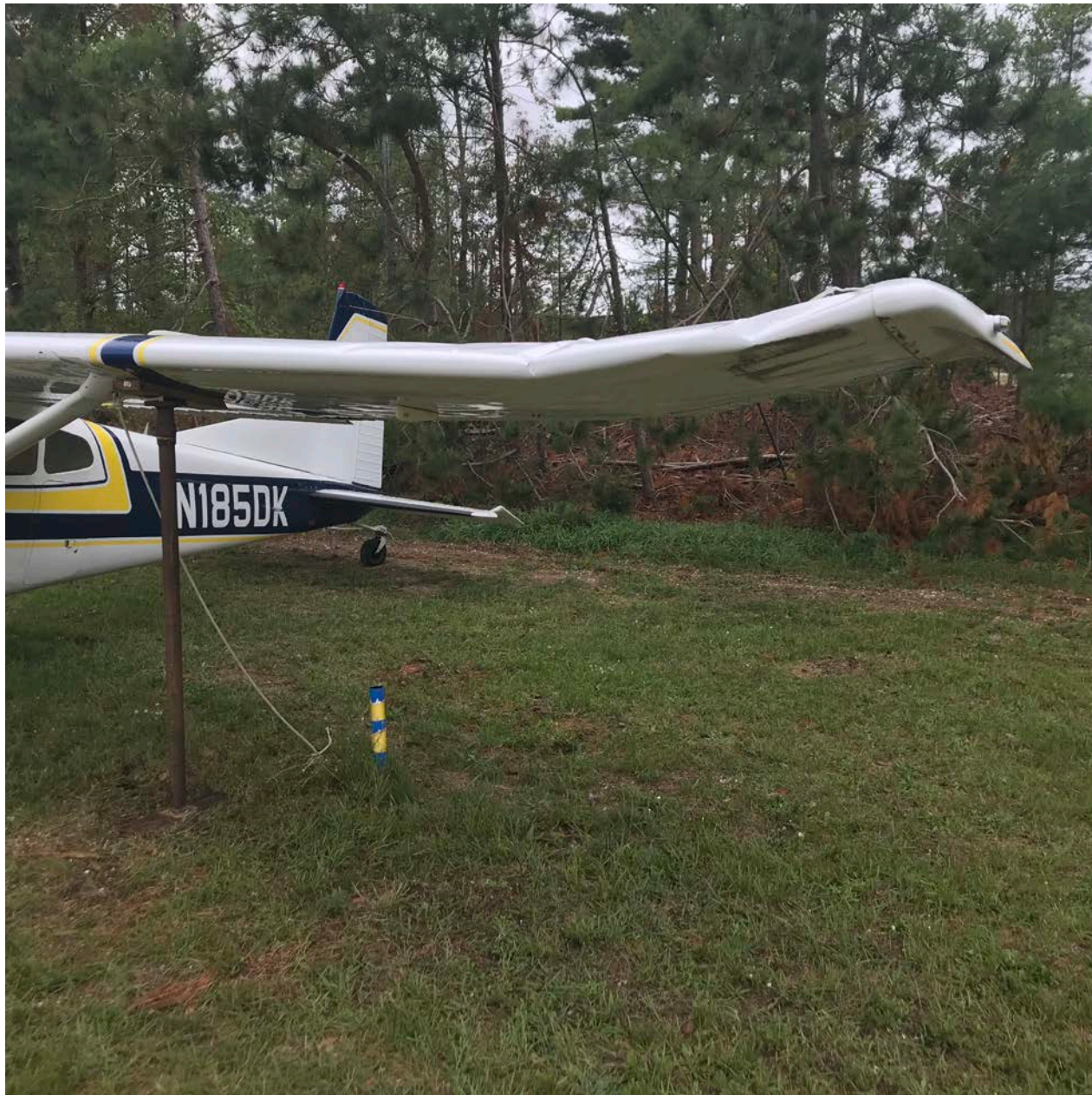
FAA Photo of Damage to Left Wing
