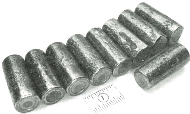
FIGURE 11 TYPICAL APPEARANCE OF ROLLERS FROM OUTBOARD CONE OF BEARING 6-3-L.
