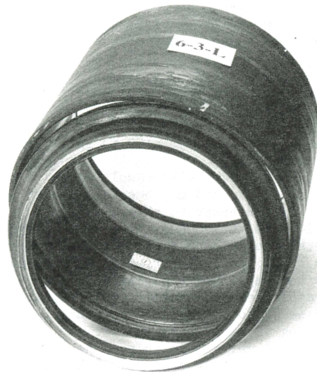
FIGURE 12 CUP AND FRONT SEAL OF BEARING 6-3-L.
