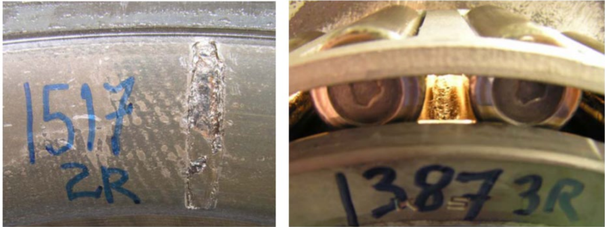
Figure 3-4. A cup fault (left) and cone fault (right) identified by RailBAM ® detectors
