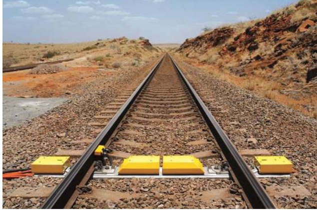
Figure 3-11. An example of HBD system (outer detectors) combined with HWD system (inner detectors) [41]
