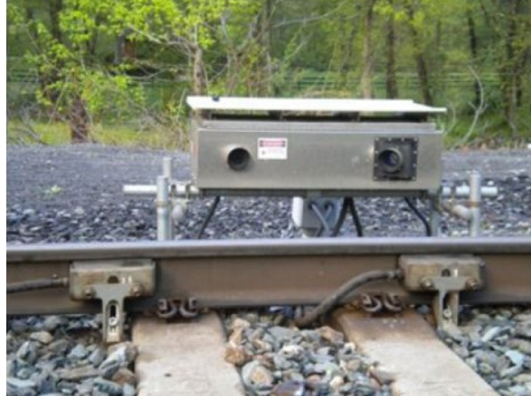
Figure 3-13. TBOGI system to identify poorly performing trucks [8]
