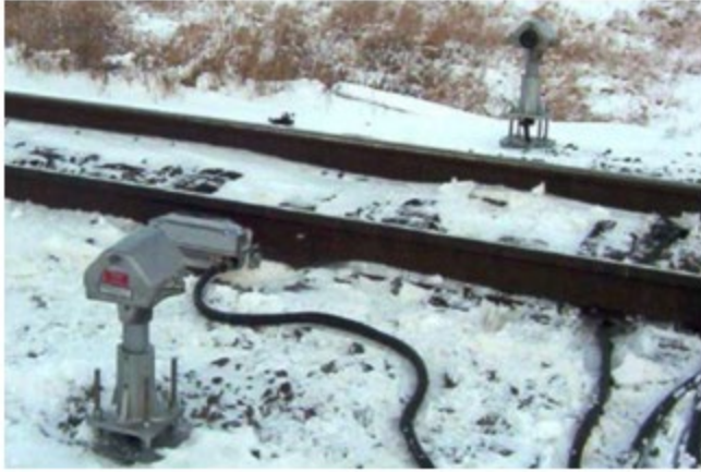
Figure 3-25. An example of WTD for brake effective tests (left); (right) Wheel temperature variation on a train indicating braking condition [8]
