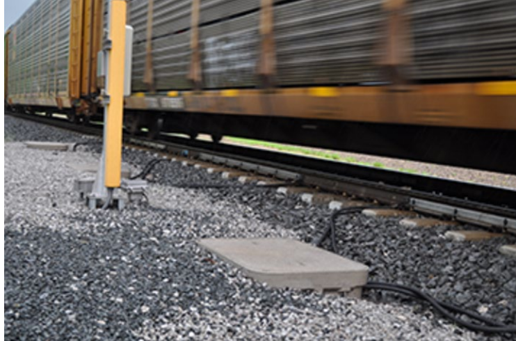
Figure 3-16. THD system based on strain-gage detectors [6]
