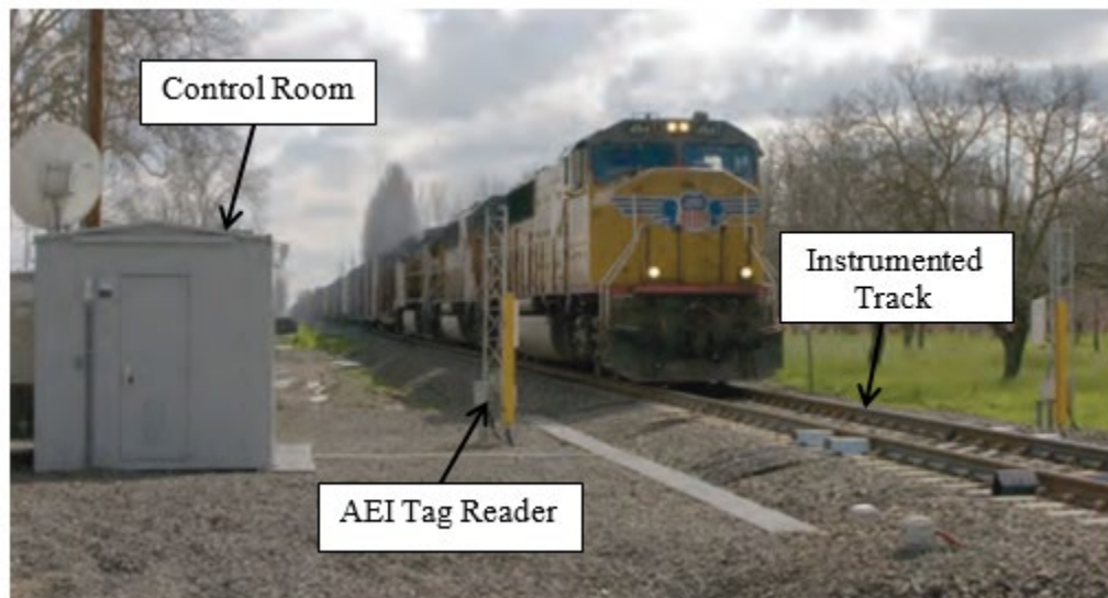
Figure 4-3. An example of WILD site components developed by L.B. Foster [59]
