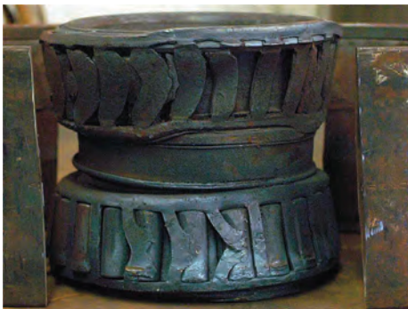
Fig. 46 Damage from a spun cone bearing failure. All internal components were fused together
