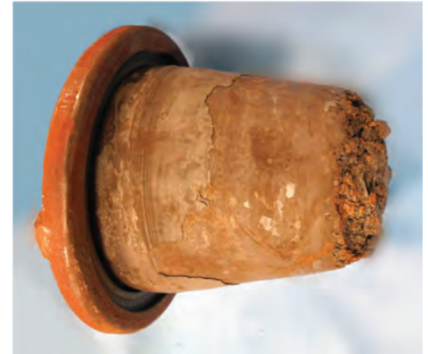
Fig. 41 Burned-off journal stub. The short, rough stub indicates high heat over a short time period and is associated with an inner cone failure
