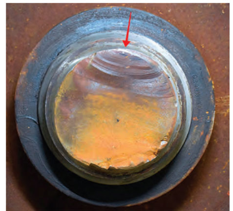
Fig. 14 Fracture surface of subject journal, axle side (arrow indicates initiation location)
