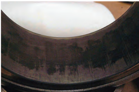
Fig. 45 Fretting wear on the inside diameter of a bearing with a spun cone
