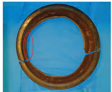
Fig. 51 As-received rim sections viewed from the back rim face. Circled area indicates initiation region
