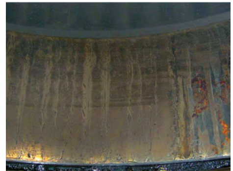
Fig. 49 Water etching with microcracking present on the cup of a bearing
