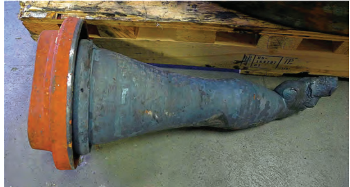
Fig. 42 Burned-off journal stub. The long, thinned-out journal indicates that the bearing was hot over a long time period and is associated with an outer cone failure
