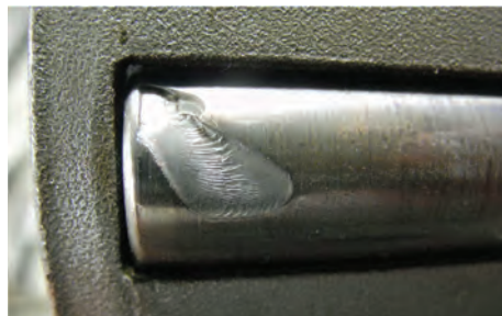
Fig. 43 Tapered roller bearing fracture from end loading due to loss of lateral clamp force
