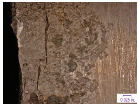
Fig. 39 Secondary fatigue cracks present near primary fracture surface
