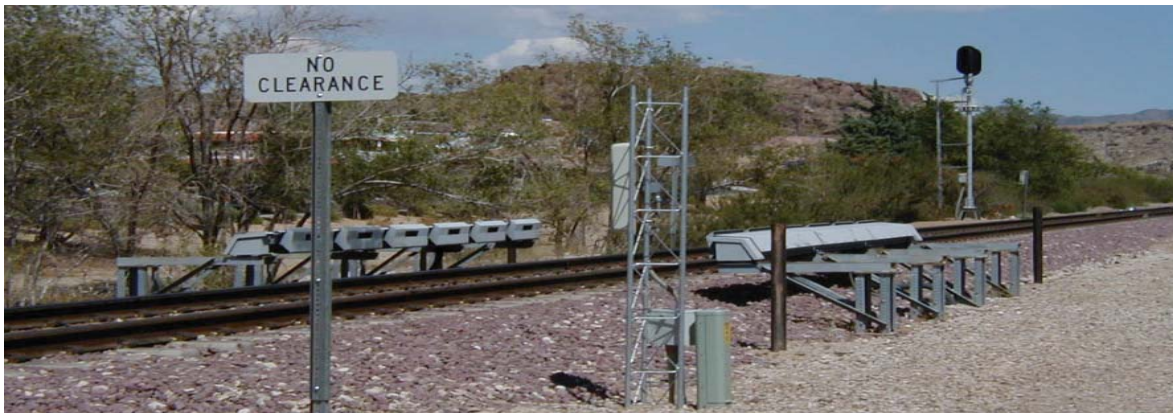
Figure 9: A Typical TAD Site in Revenue Service consisting of Microphone Array, Wheel Sensors and AEI
