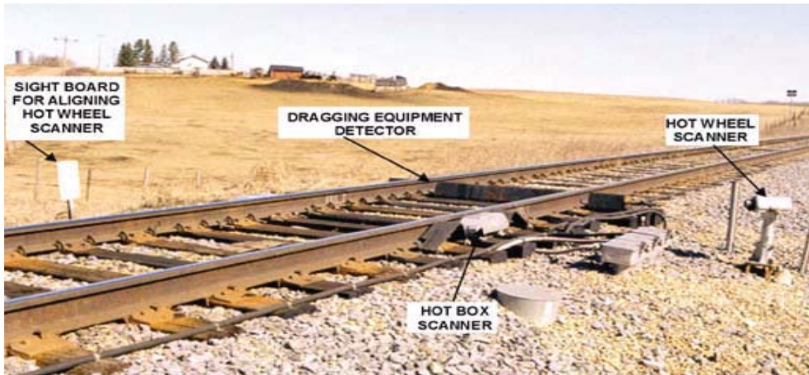
Figure 19: A Super Site on Revenue Track showing HWD, HBD and DED. The HWD has only One Scanner at an Angle to the Track with a White Reference Board on the Far Side.
