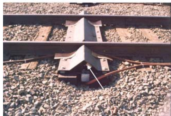
Figure 17: Impactor style DED showing location of an accelerometer on the underside of the strike plate
