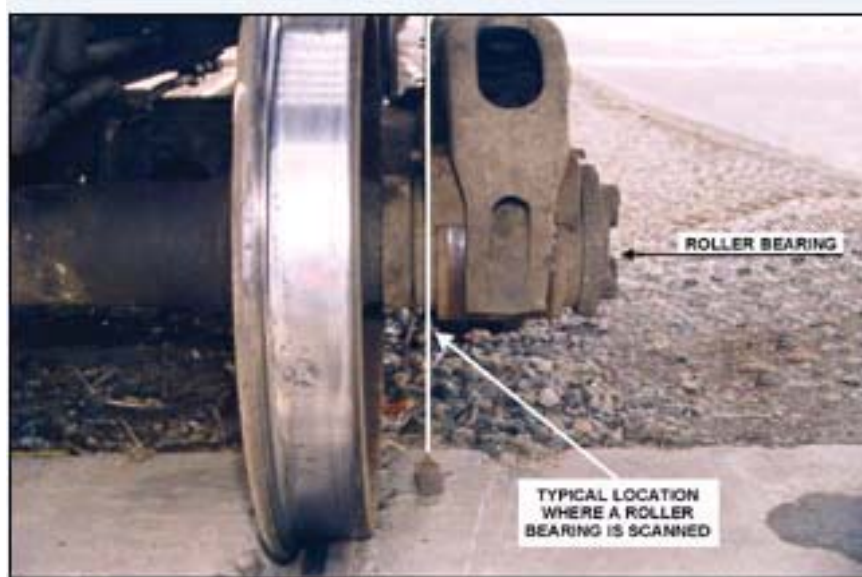
Figure 14: Typical Location for Scanning a Bearing
