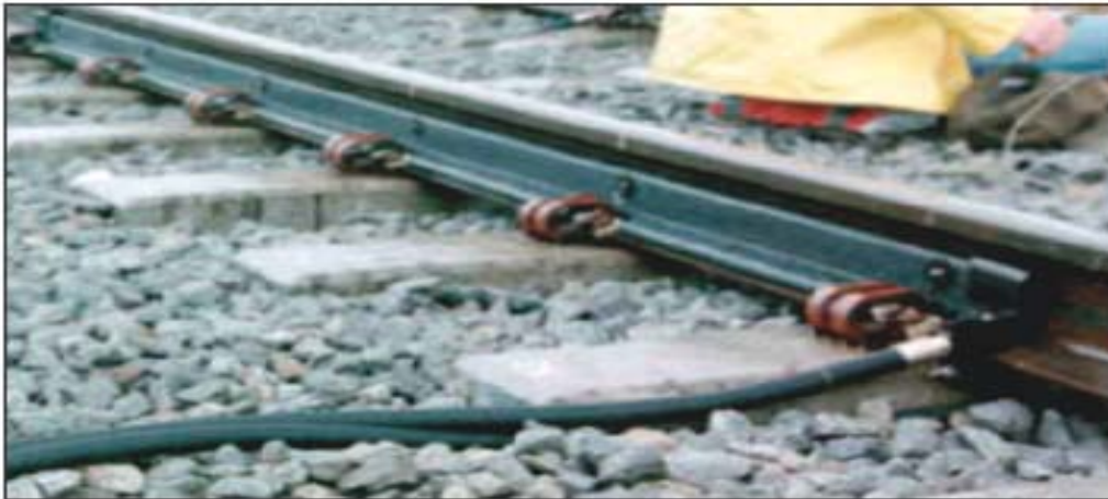
Figure: 21: Shown LIOD consists of an Angle Iron bolted to Rail at every Tie Location and also anchored with Rail to Ties with Elastic Clips. The Angle Iron is instrumented on Crib Locations to measure Wheel Loads. As shown, the LIOD can be detached and anchored as needed.
