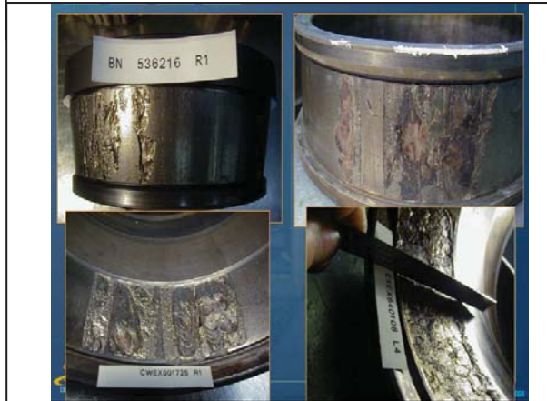
Figure 7: Damaged Cups and Cones of Bearings
