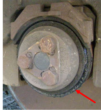
VISIBLY LEAKING BEARING WITH CLEARLY FORMED DROPLETS
