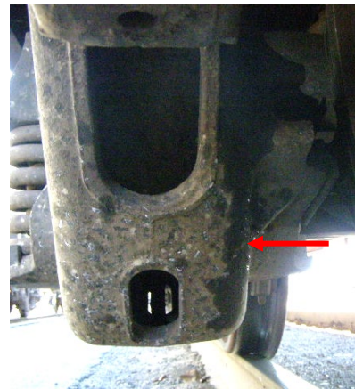
BEARING LEAK INDICATION - SLUNG GREASE
