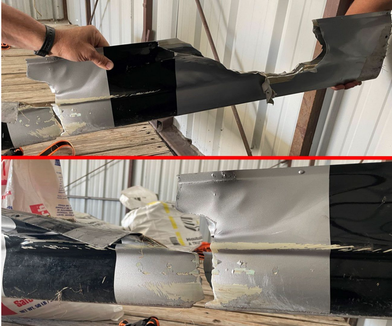
Photograph 1. Separated outboard sections of the helicopter's main rotor blades.
