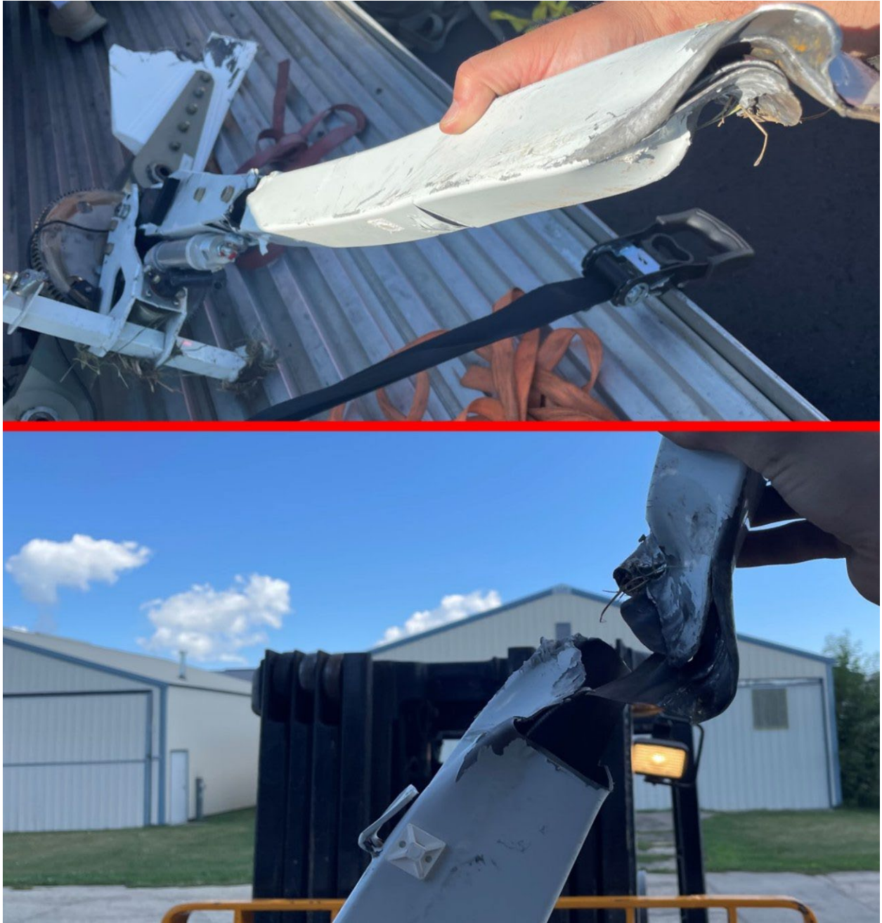
Photograph 3. Gyroplane's separated rotor mast section and the helicopter's main rotor blade contact witness mark.
