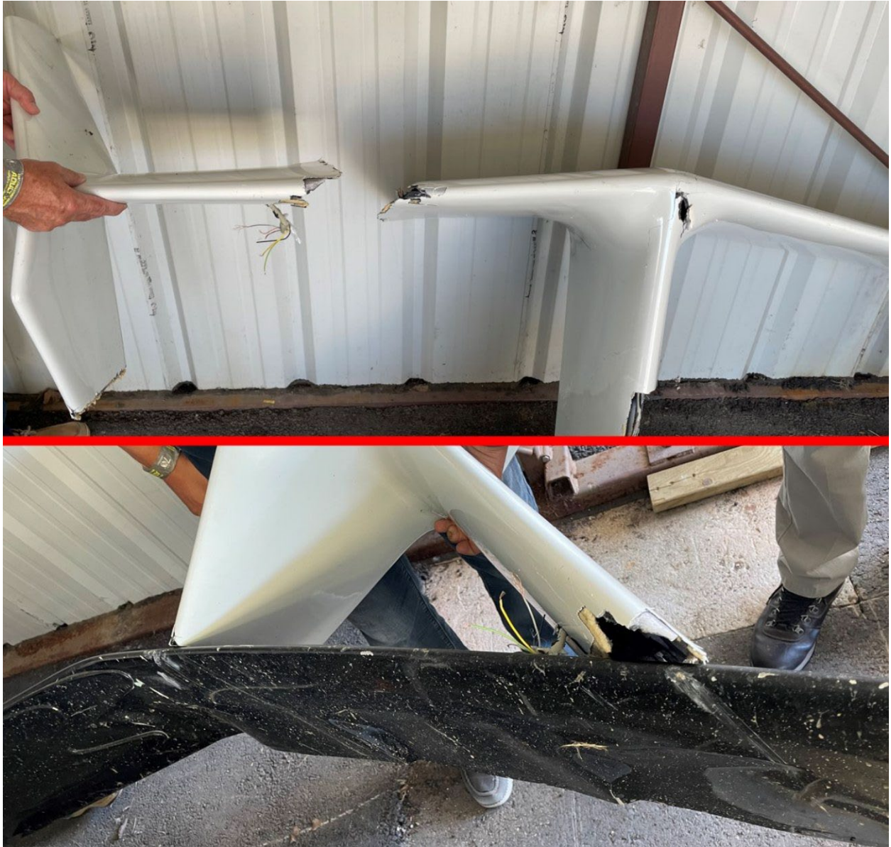
Photograph 2. The upper photograph depicts the gyroplane's separated right horizontal stabilizer and lower vertical stabilizer. The lower photograph depicts the separated stabilizer section in comparison with the helicopter main rotor blade contact witness marks and white paint transfer.
