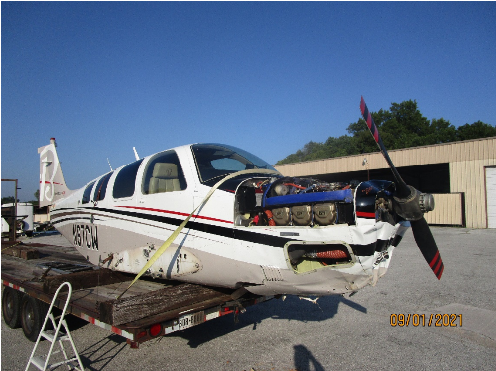
Airplane strapped down to trailer, for the engine run, with a replacement propeller installed
