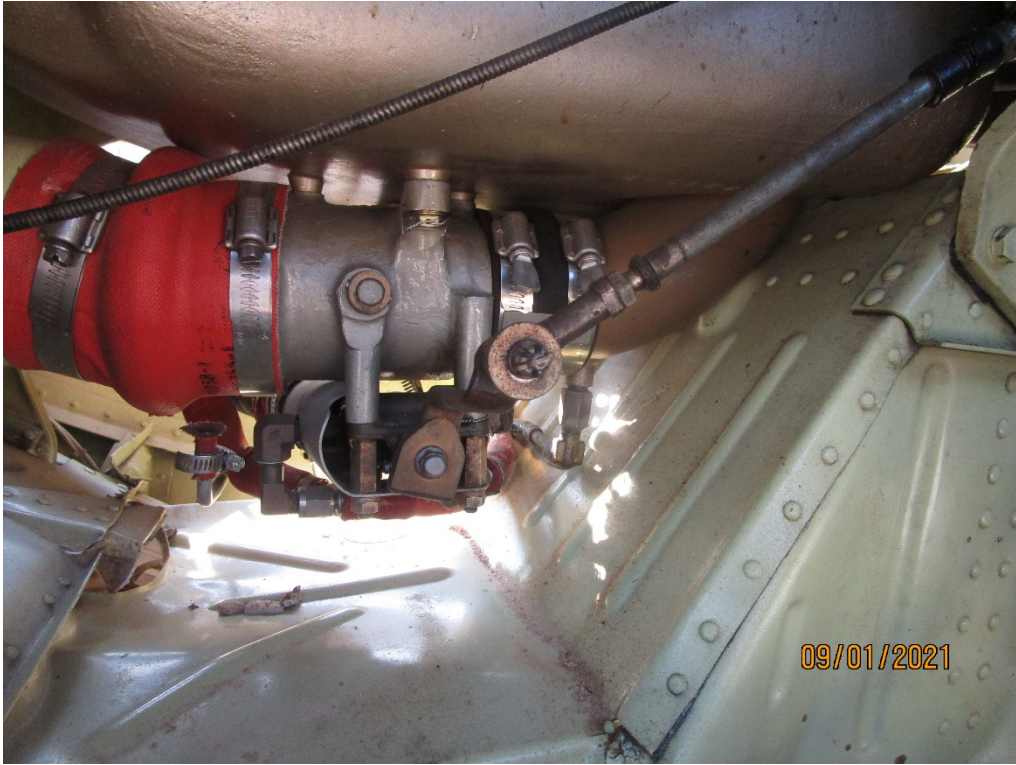
Throttle body; engine controls connected.
