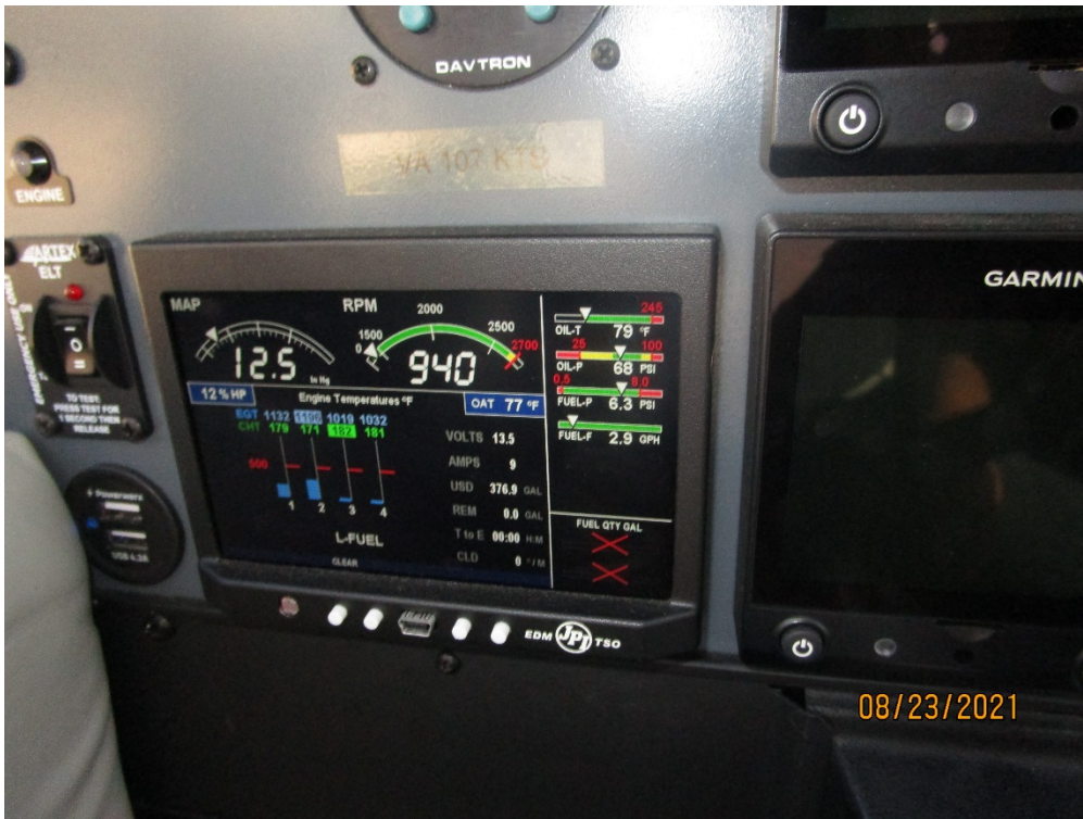
Engine monitor during the engine test run
