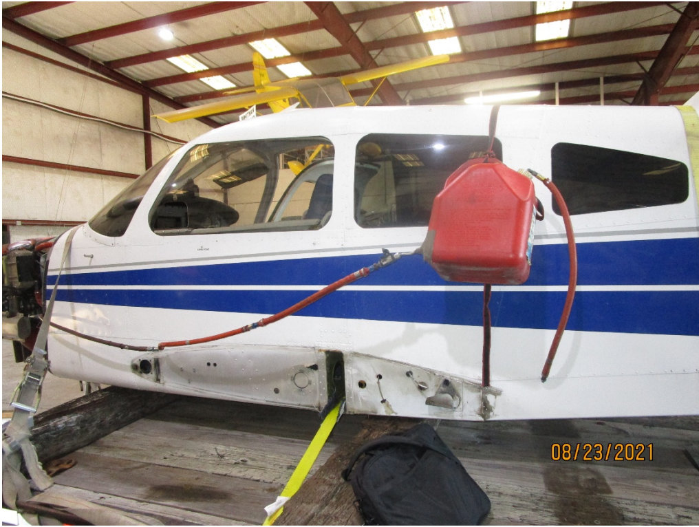
Fuel can, plumbed to the engine
