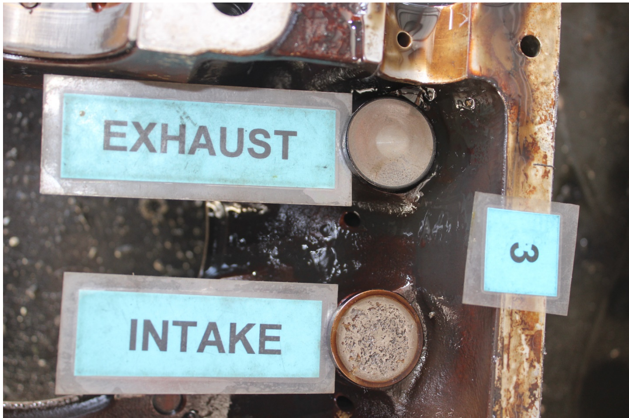
Photo 12: No 3 Exhaust and Intake tappets
