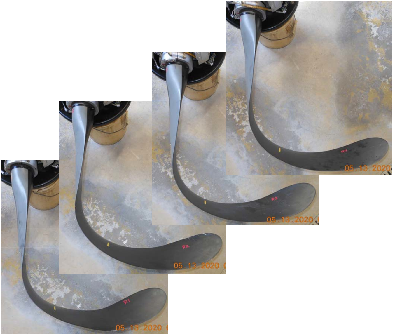
Photo #12 – Right propeller blades relative bend and twist (R1-R4 left-to-right)
