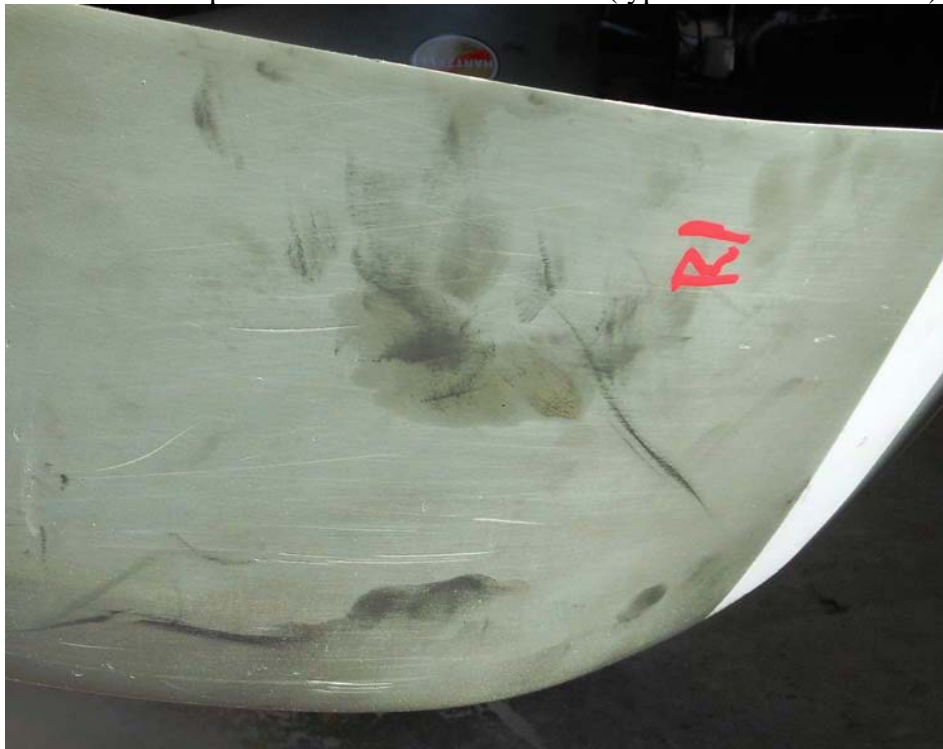
Photo #14 – Spanwise abrasion in mid-blade (typical of all four blades)
