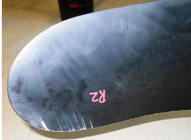
Photo #13 – Chordwise/rotational scoring on R2 face side
