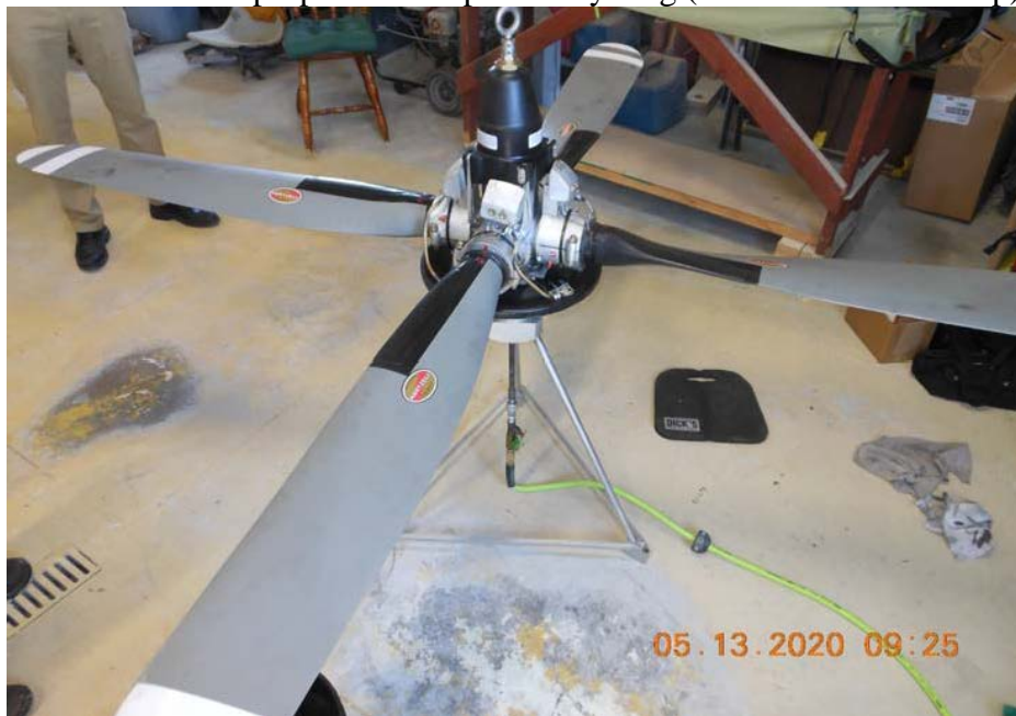
Photo #6 – Left propeller on tripod for cycling (shown on reverse stop)
