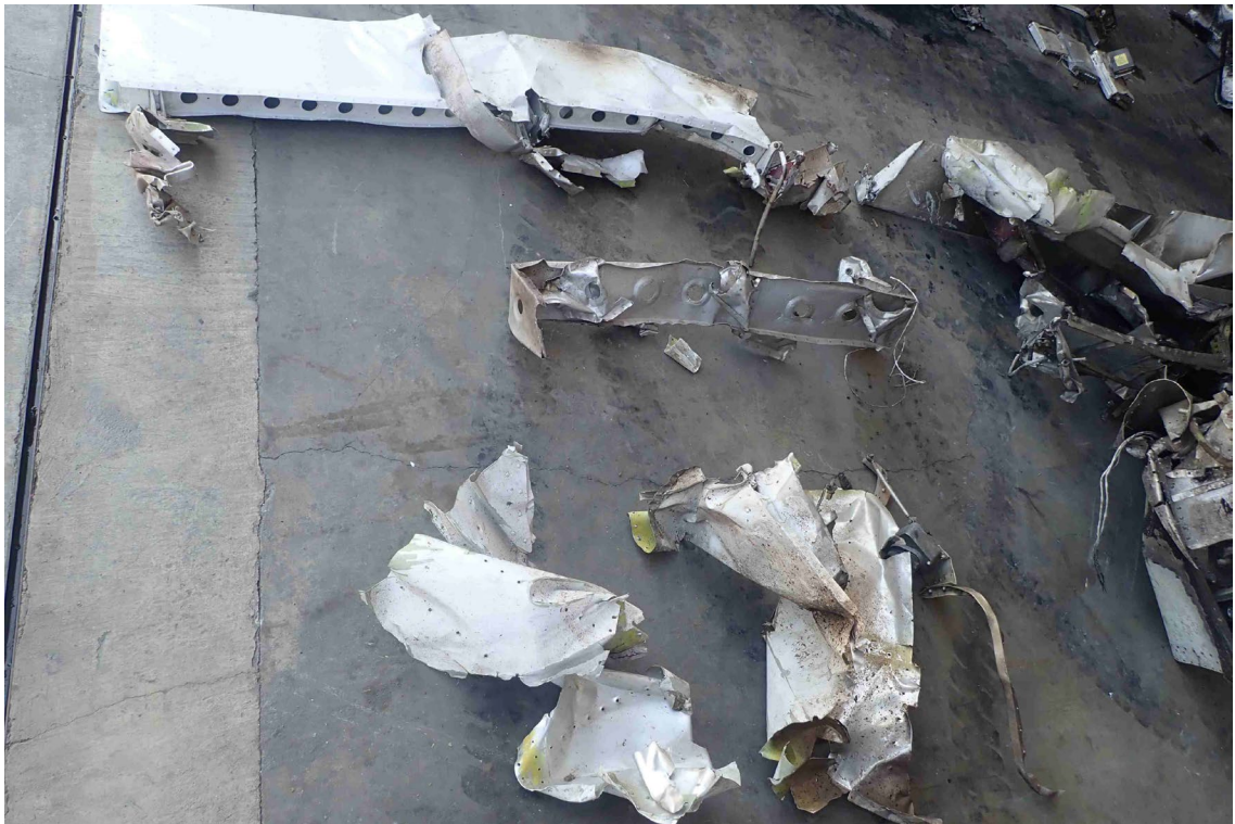
Figure 20- Outboard left wing fragments
