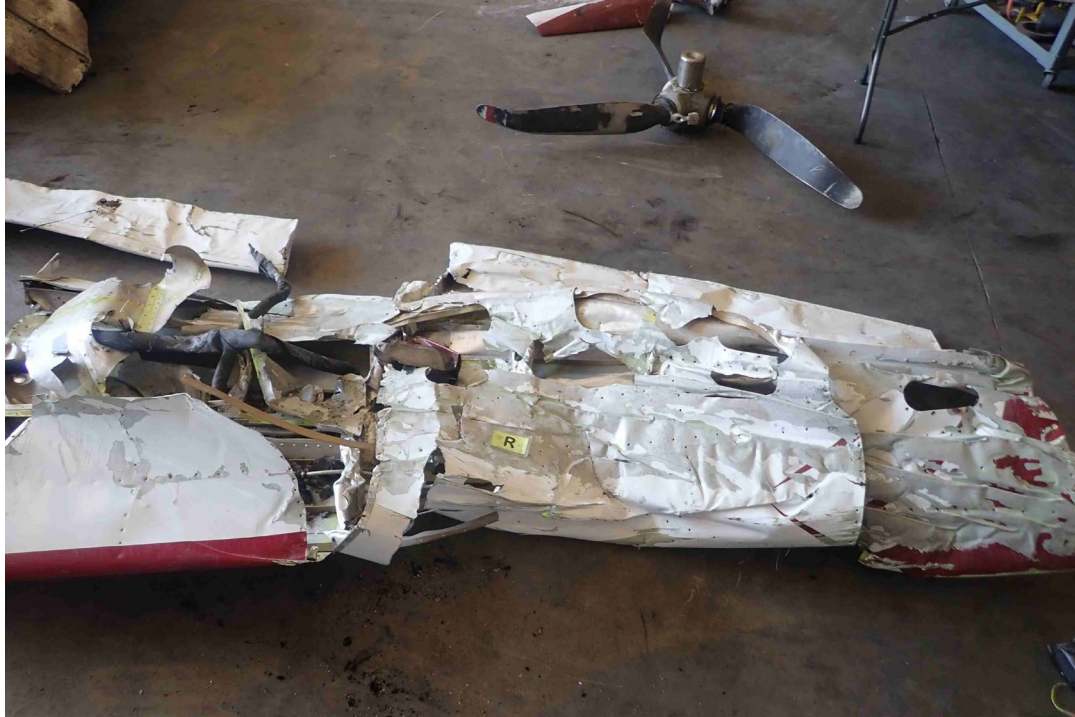
Figure 14 - Outboard right wing
