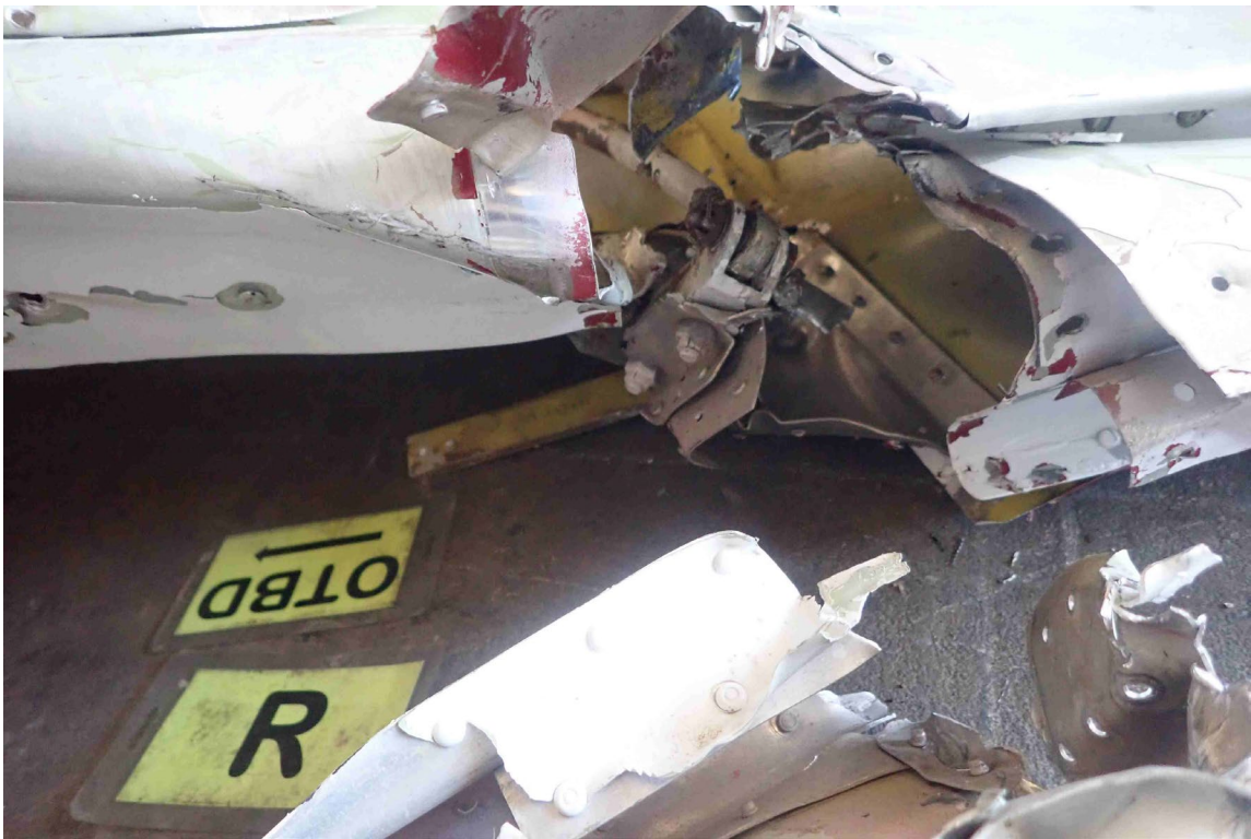
Figure 16 - Inboard right aileron hinge
