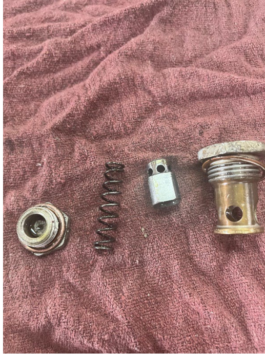
Figure 6: Disassembled oil pressure relief bypass valve. Photo courtesy of Anderson Aeromotive Inc.
