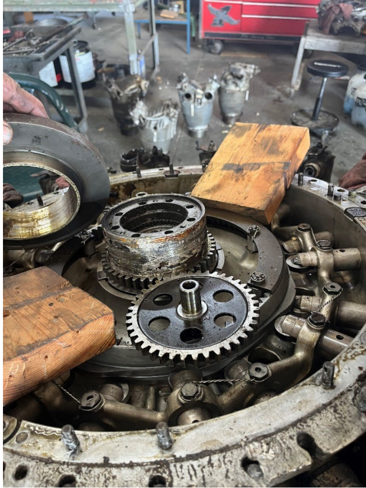
Figure 11: Rear counterbalance, rear counterbalance bearing, and rear cam. Photo courtesy of Anderson Aeromotive Inc.
