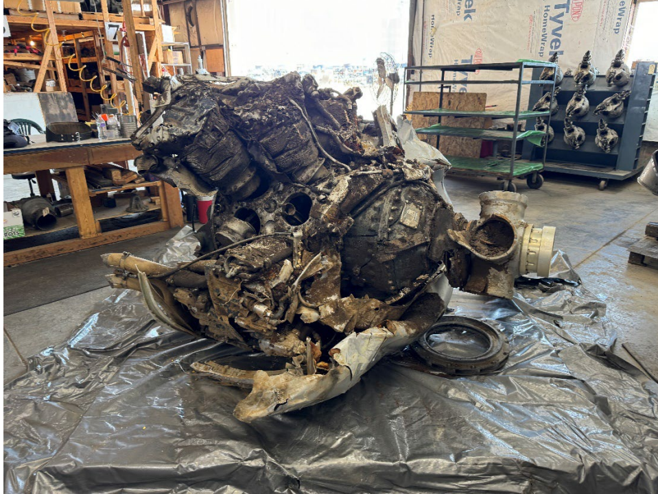
Figure 3: Forward section of the engine with the area of impact damage and displaced cylinders.
