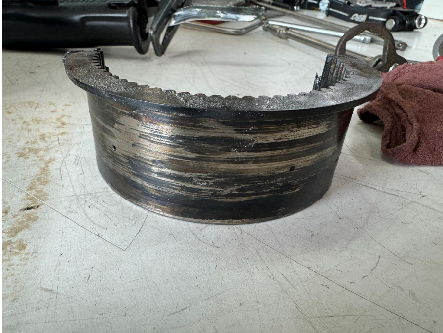
Figure 9: Portion of the front secondary counterbalance bearing.
