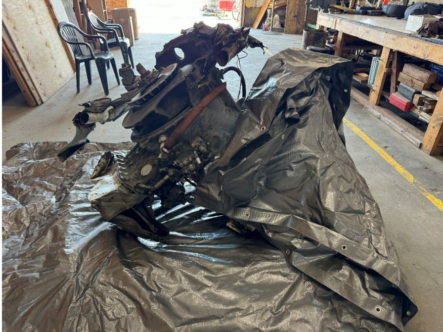
Figure 2: Collector case, intermediate rear case, and rear case assemblies.
