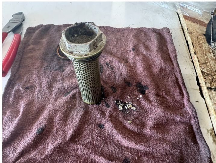
Figure 4: Intermediate rear case scavenge oil screen and metallic flakes.
