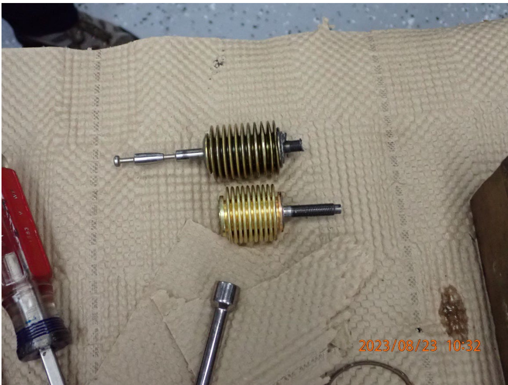
Photo 4: Exemplar aneroid bellows (lower) vs aneroid bellows from accident engine (upper).
