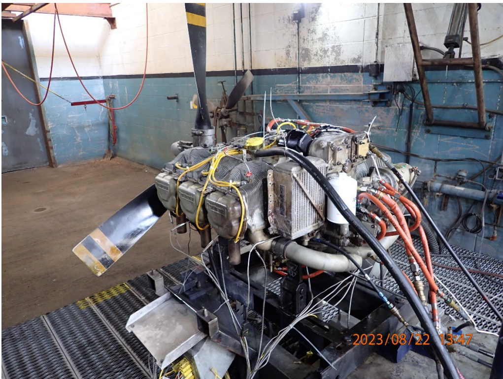
Photo 2: The engine fitted to the stand for test run.
