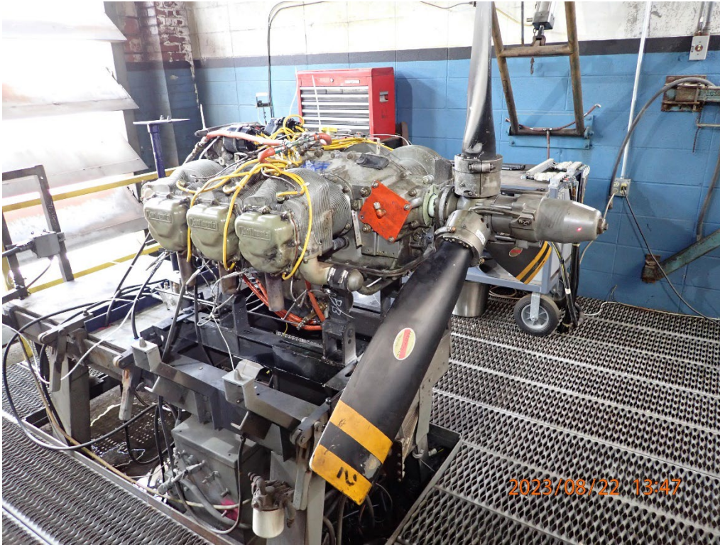
Photo 3: The engine fitted to the stand for test run.
