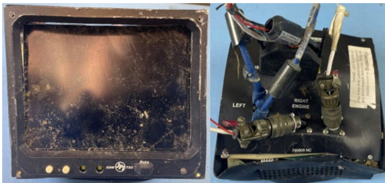
Figure 1. Front (left) and back (right) of JPI EDM-960 as received by the NTSB Vehicle Recorder Laboratory.
