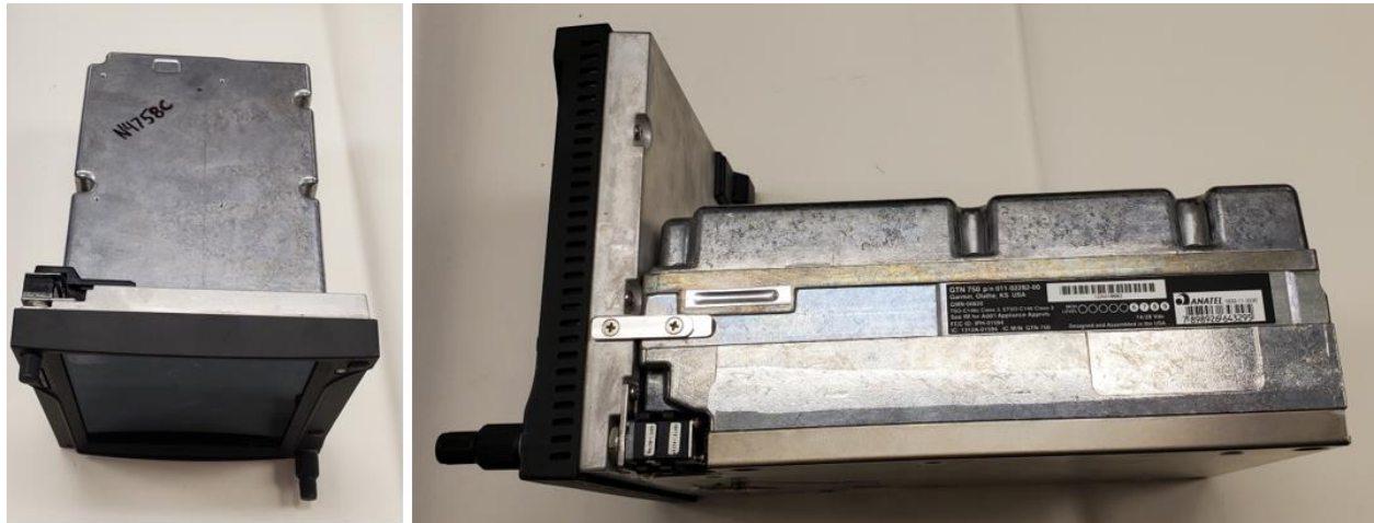
Figure 2. Top and side views of the Garmin GTN 750 as received.
