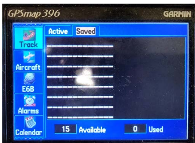
Figure 4. Garmin GPSMAP 396 “Track” screen showing that no track logs were recorded to NVM.
