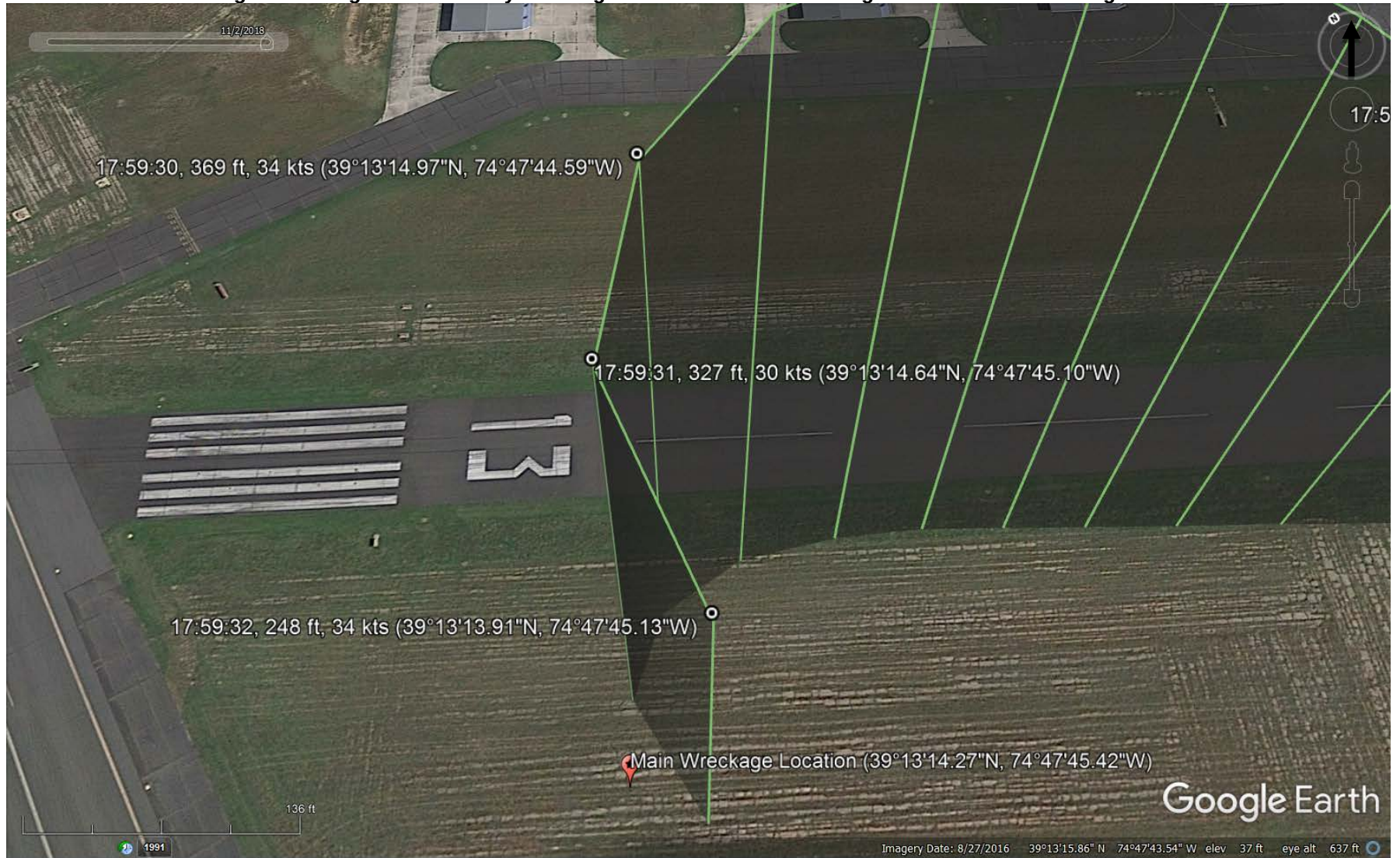
Figure 9. Google Earth overlay showing the end of the accident flight and the main wreckage location.
