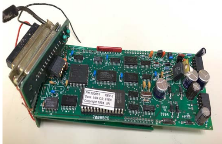
Figure 2. Internal components of JPI EDM-700. No presence of non-volatile memory.
