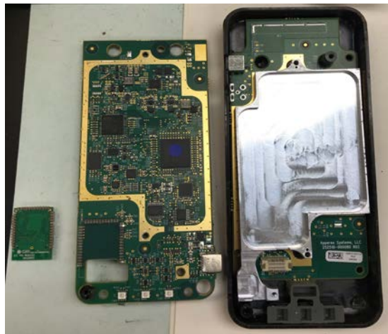
Figure 2. Dislodged and broken internal components of the Appareo Stratus 3i.
