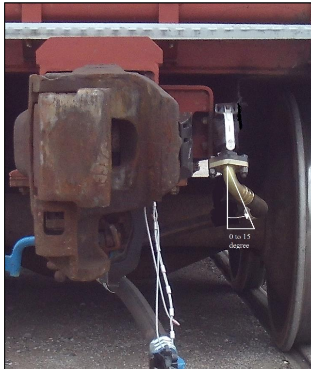
Figure 3: Example of Sweep Elbow Orientation (The intermediate hose should point outboard 0-15 degrees from longitudinal centerline of car)
