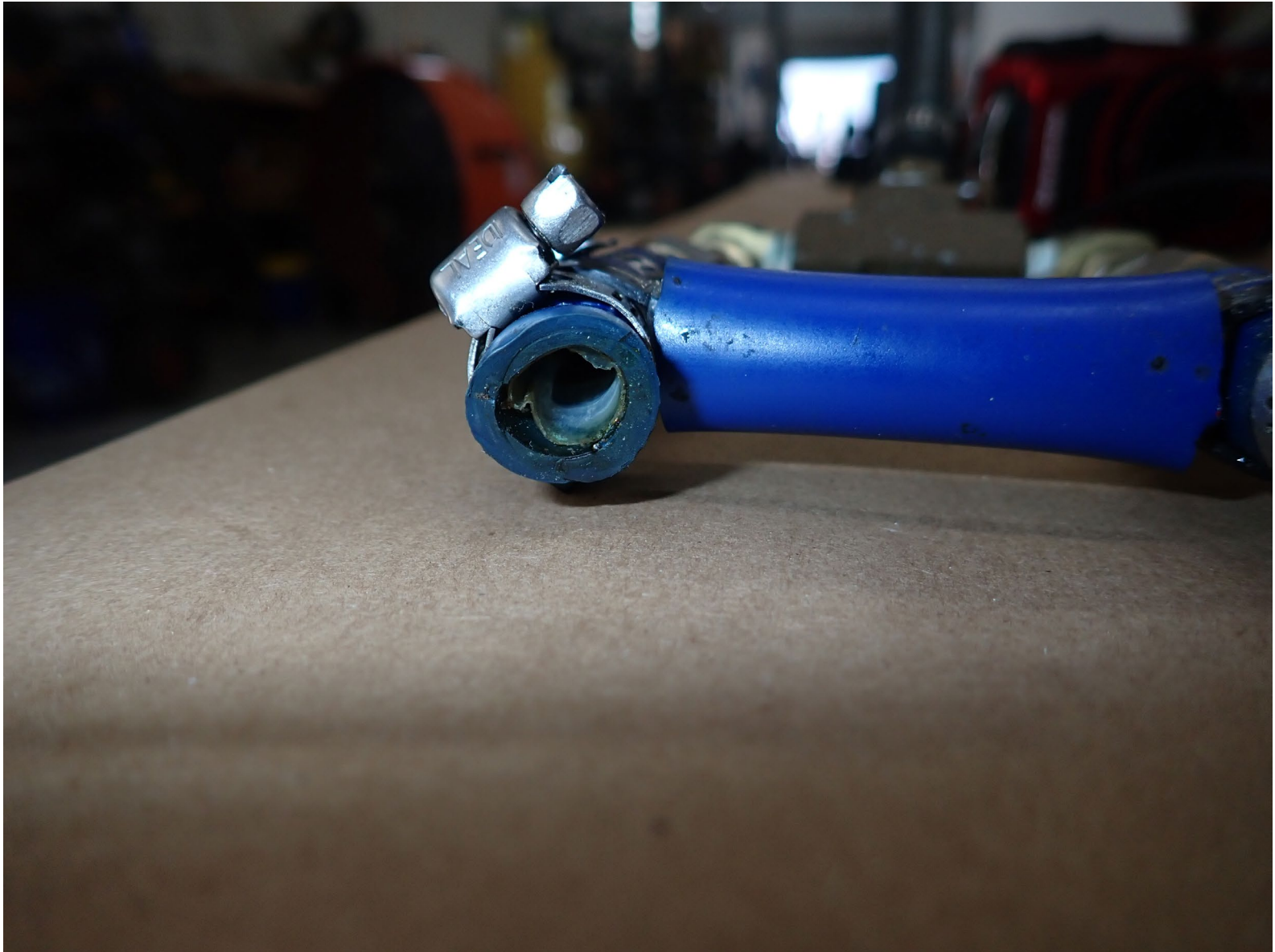
Photograph 6 - Partially occluded fuel hose from fuel pump outlet manifold
