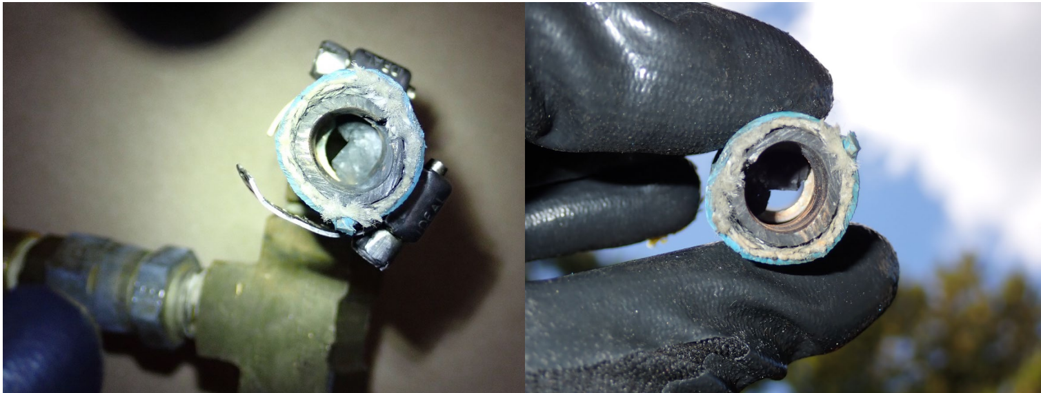
Photograph 3 & 4 - Two views of partially occluded fuel line from fuel pump inlet manifold
