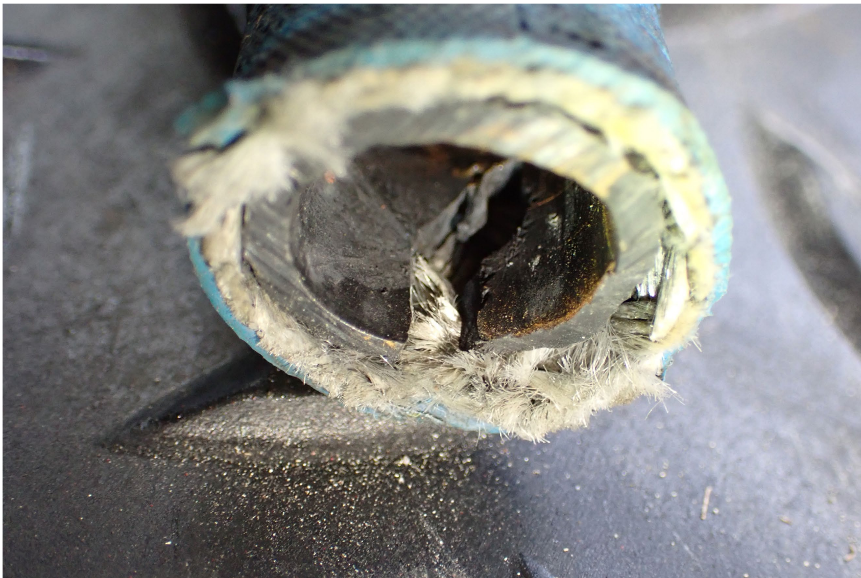
Photograph 4 - Cracked fuel hose from fuel pump inlet manifold
