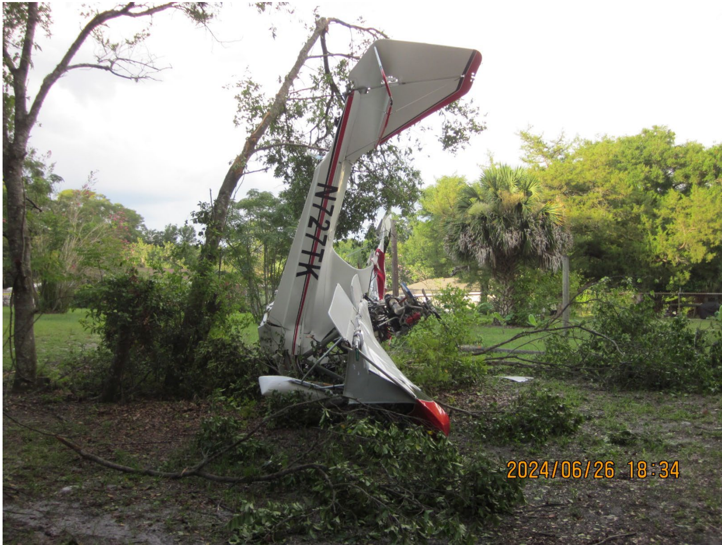
Photograph 2 - Postaccident view of wreckage (Courtesy of FAA)
