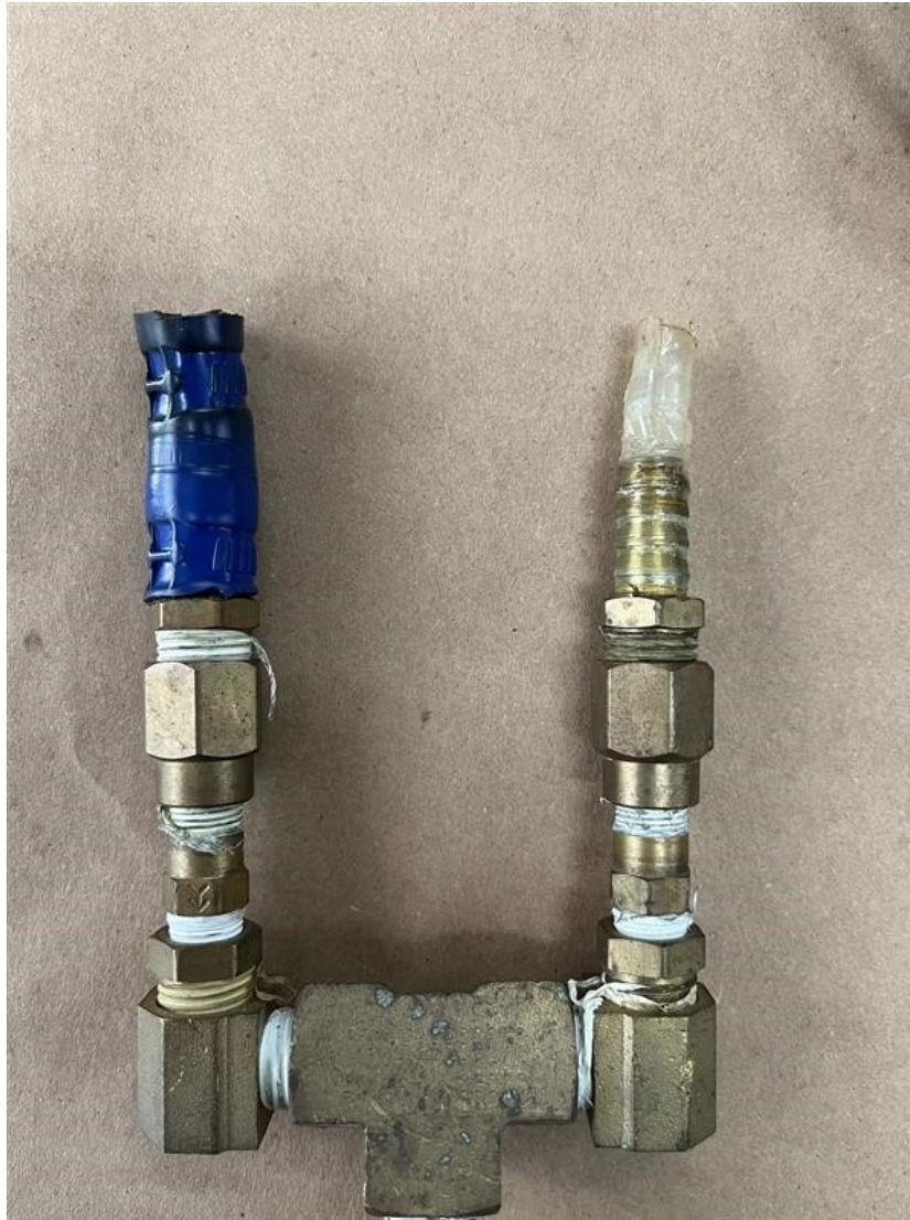
Photograph 5 - Fuel pump outlet manifold hose and fitting installation
