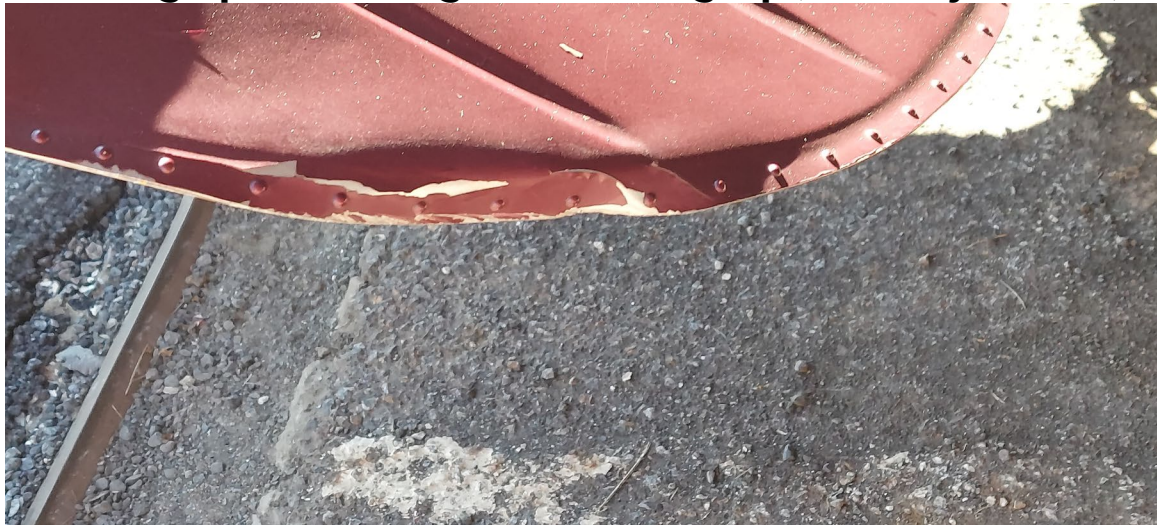
Photograph 2 - Damage to Left Elevator (Courtesy of Pilot)
