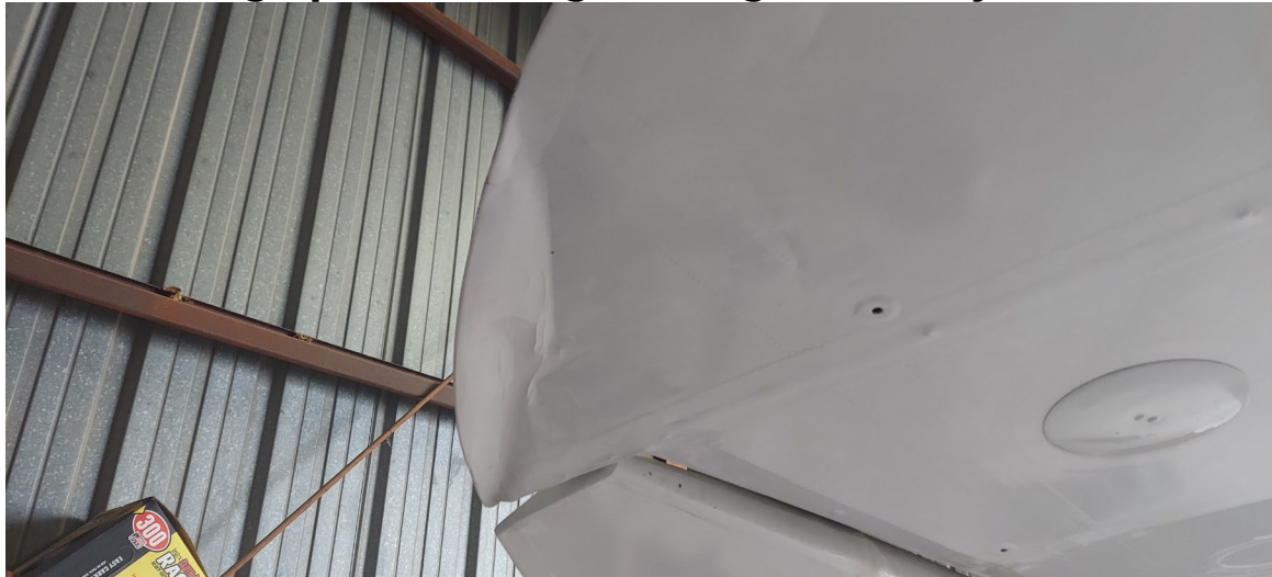
Photograph 4 - Damage to Right Wing (Courtesy of Pilot)
