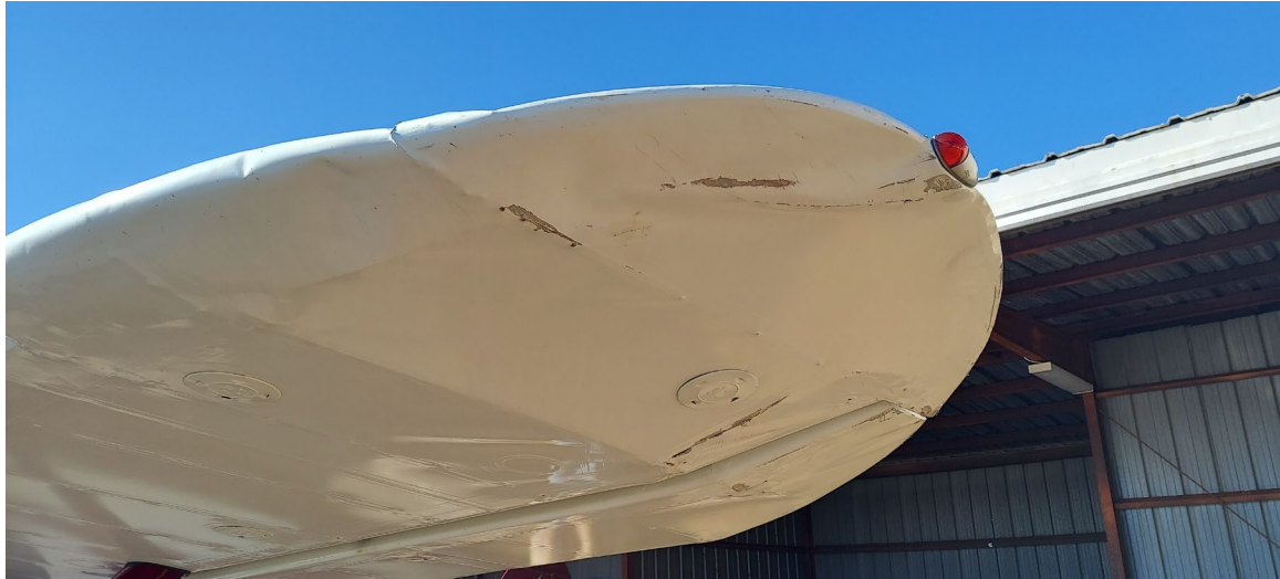
Photograph 1 - Damage to Left Wing Tip (Courtesy of Pilot)
