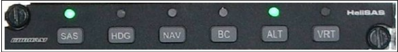
Figure 3: Exemplar HeliSAS Control Panel (HCP)
