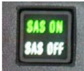
Figure 2: HeliSAS SAS ON/SAS OFF Switch
