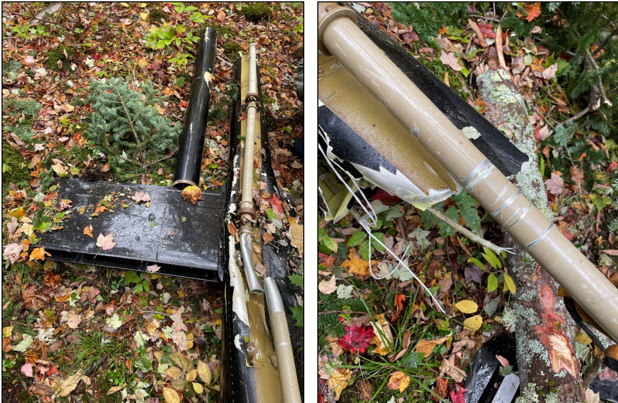
Figure 8: Views of the tail rotor drive shaft.
