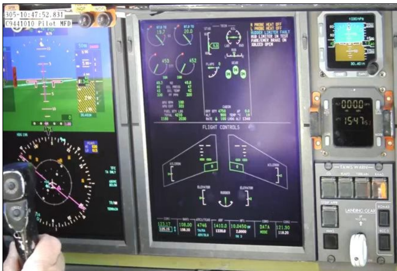
Figure 4: Screenshot taken during the STALL/ RUD LIM test.
