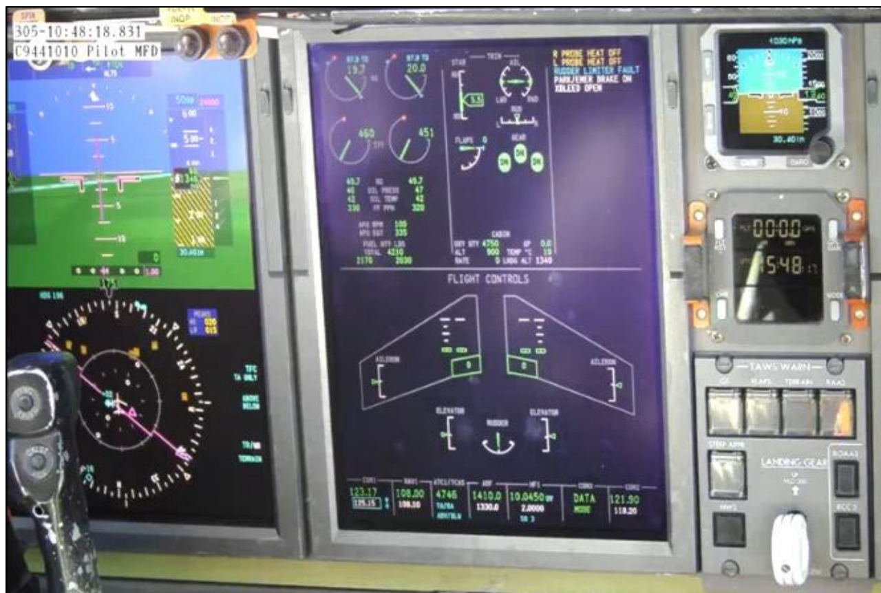
Figure 5: Screenshot taken following the conclusion of the two STALL/ RUD LIM tests, with the RUDDER LIMITER FAULT advisory CAS remaining posted.
