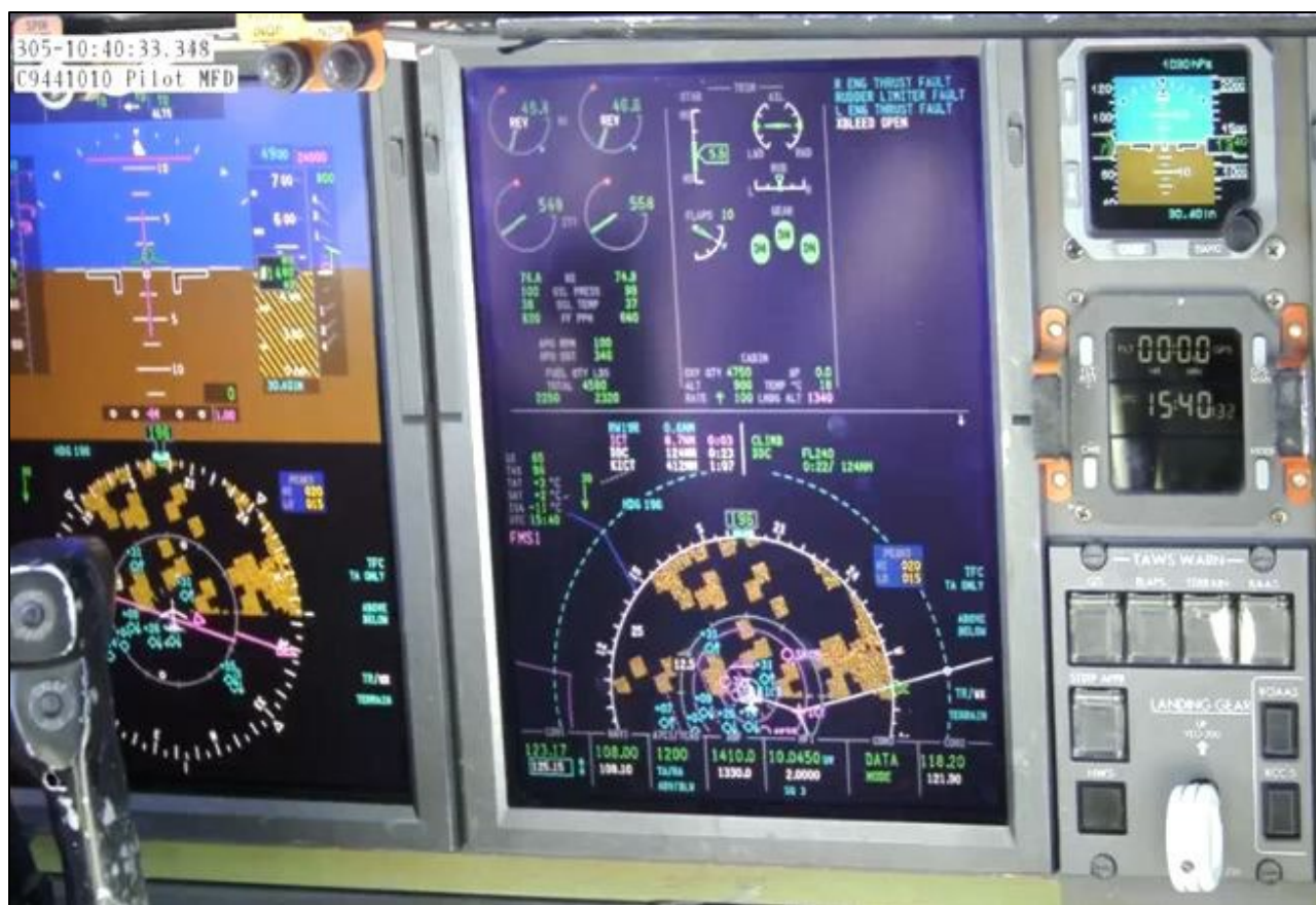
Figure 2: Screenshot taken as the crew announced 90 kts and at the moment thrust was reduced in the RTO.
