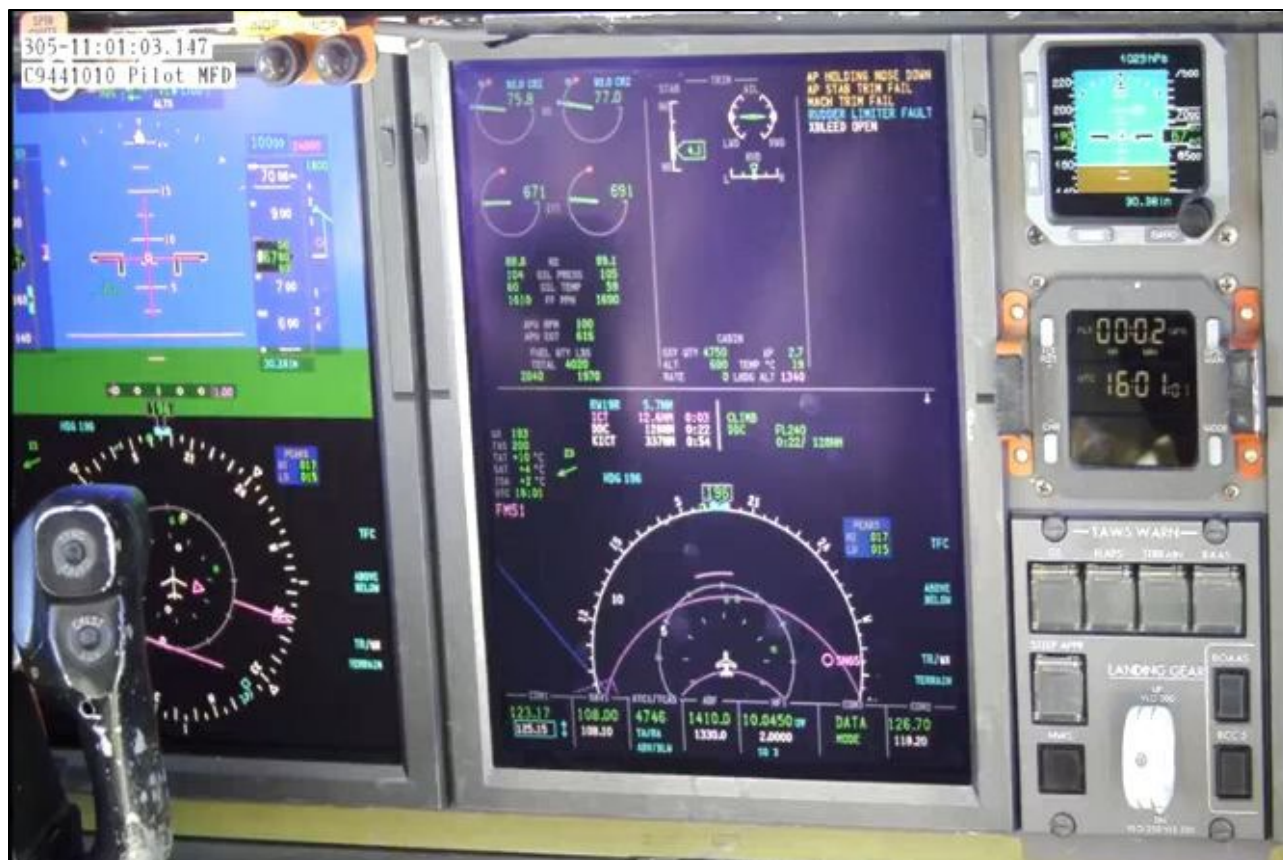
Figure 11: Screenshot taken when AP HOLDING NOSE DOWN posted.
