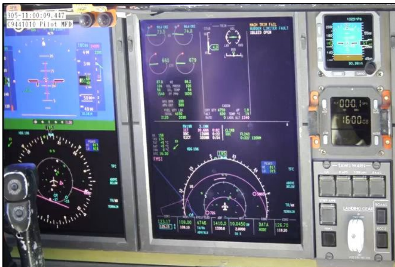
Figure 9: Screenshot following first AP disengagement.
