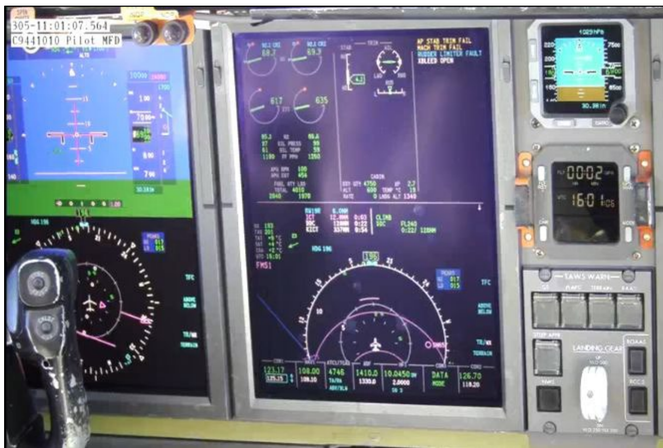
Figure 12: Screenshot taken when AP HOLDING NOSE DOWN cleared.
