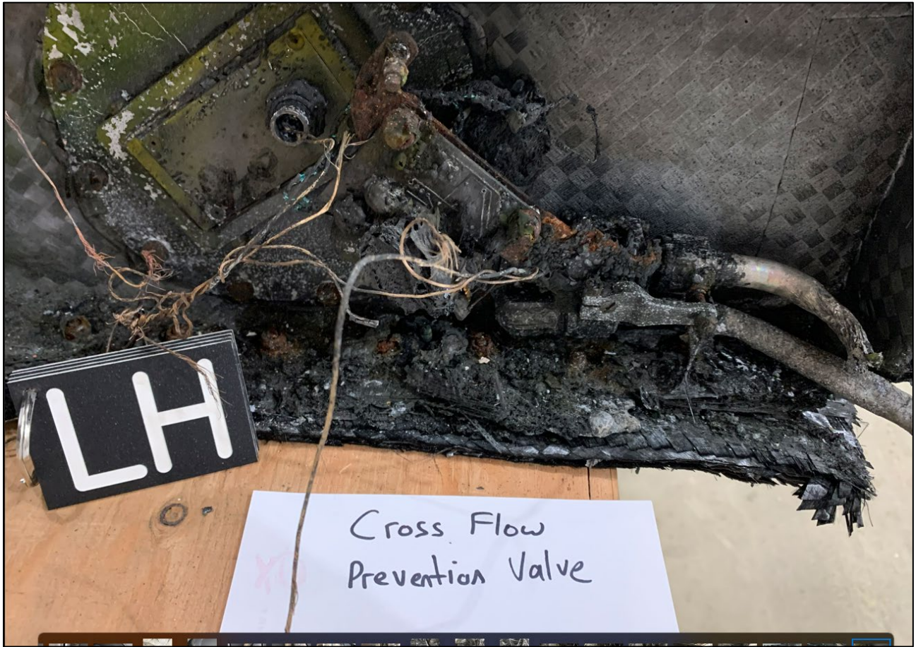
Photo 5: View of the cross flow prevention valve installed to a fragment of left wing.
