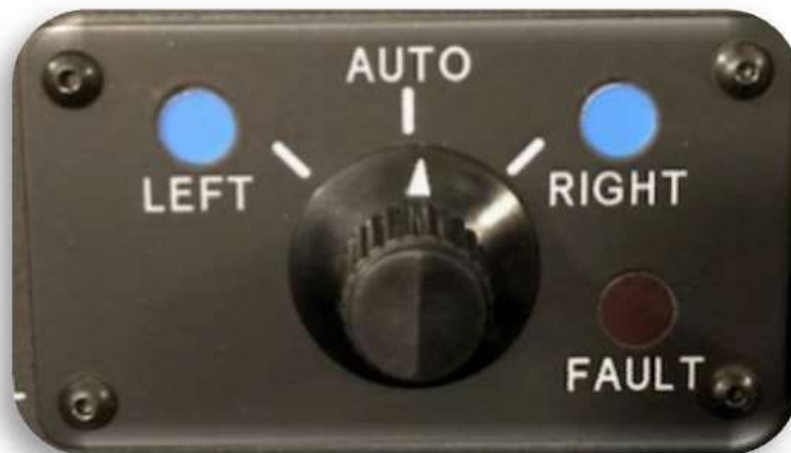
Figure 6: Photo of a fuel controller located in POH.
