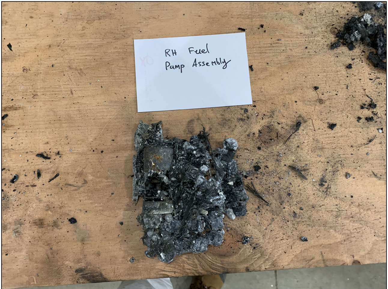
Photo 4: View of the right fuel pump assembly
