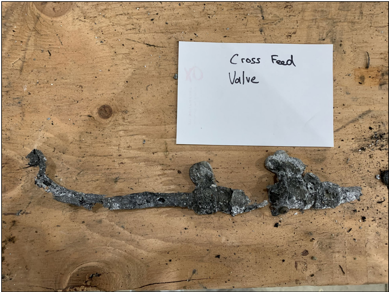
Photo 6: View of the cross feed valve recovered in the wreckage.
