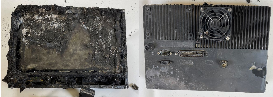
Figure 2. Front and back of the Garmin GDU 460 PFD as received.
