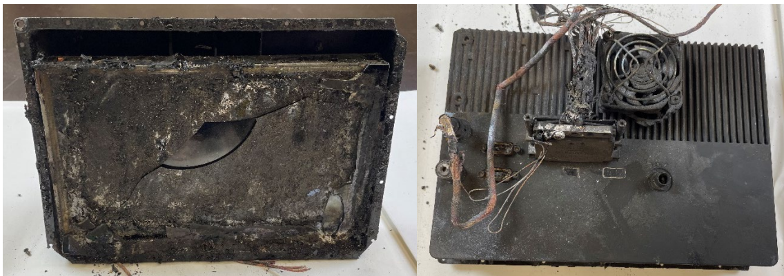
Figure 3. Front and back of the Garmin GDU 460 MFD as received.
