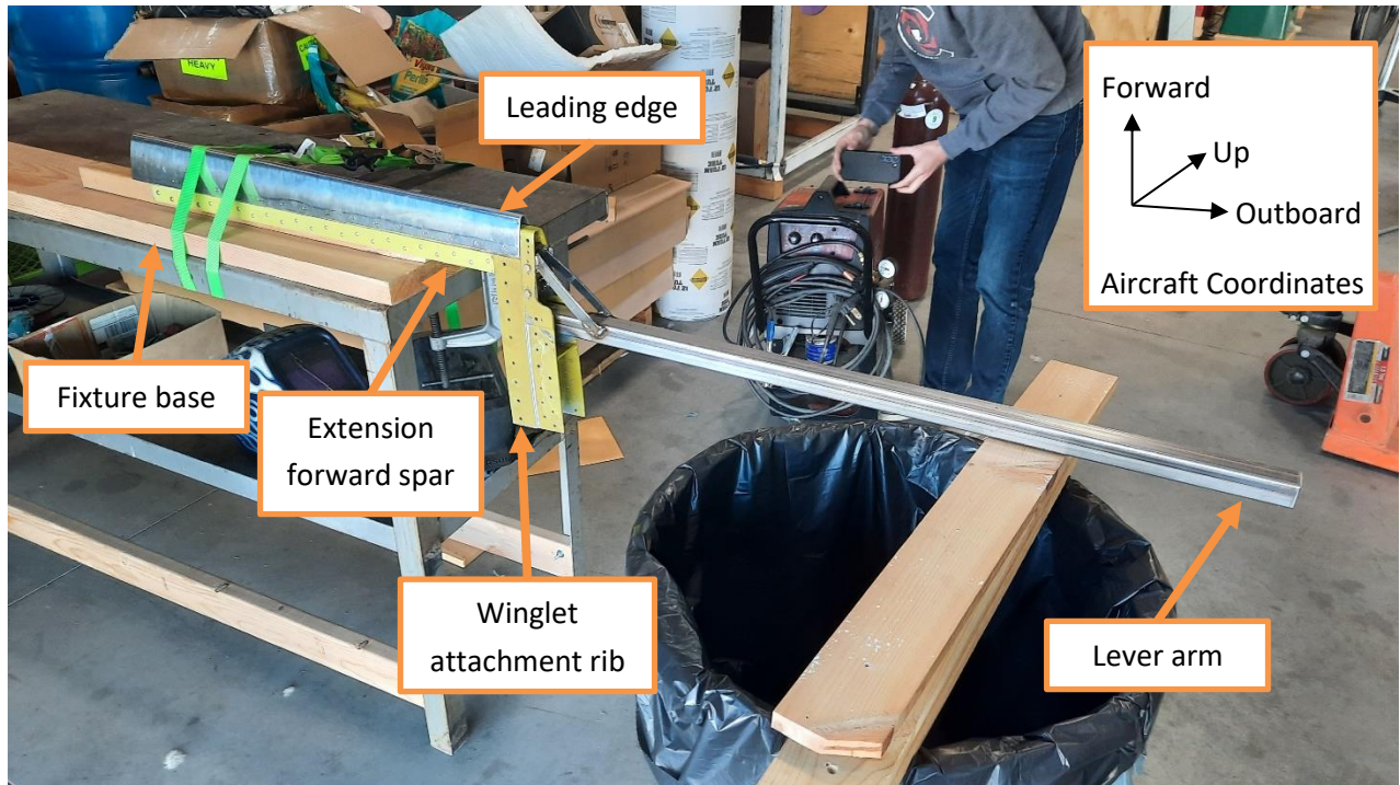
Figure 3-1 Company winglet rib tear-out test setup
