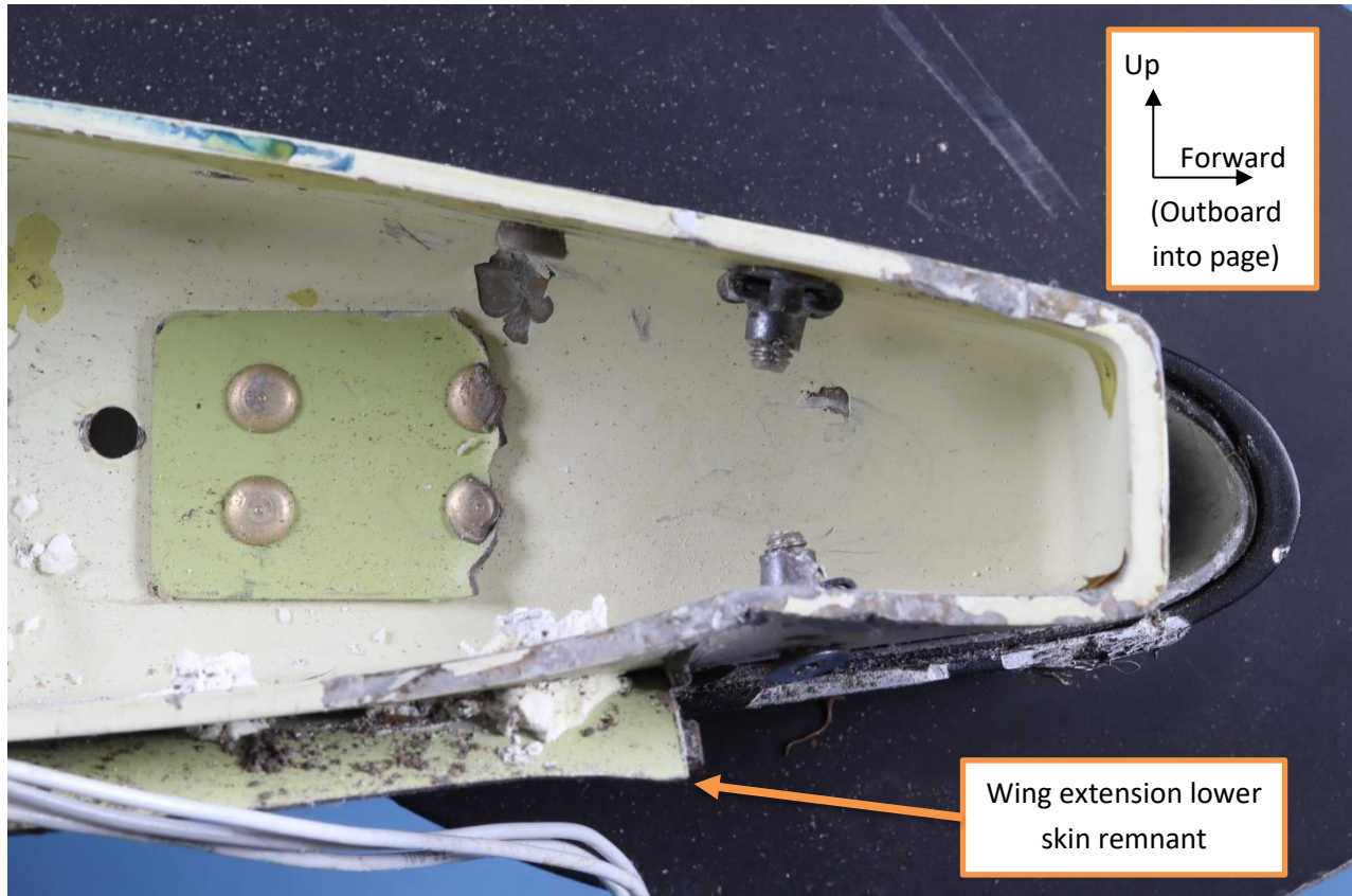
Figure 3-12 Detail view of the winglet attachment rib
