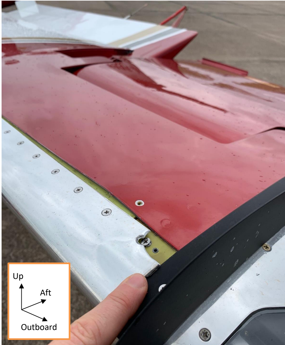
Figure 3-6 Example of confirmed ground damage (separate incident)
