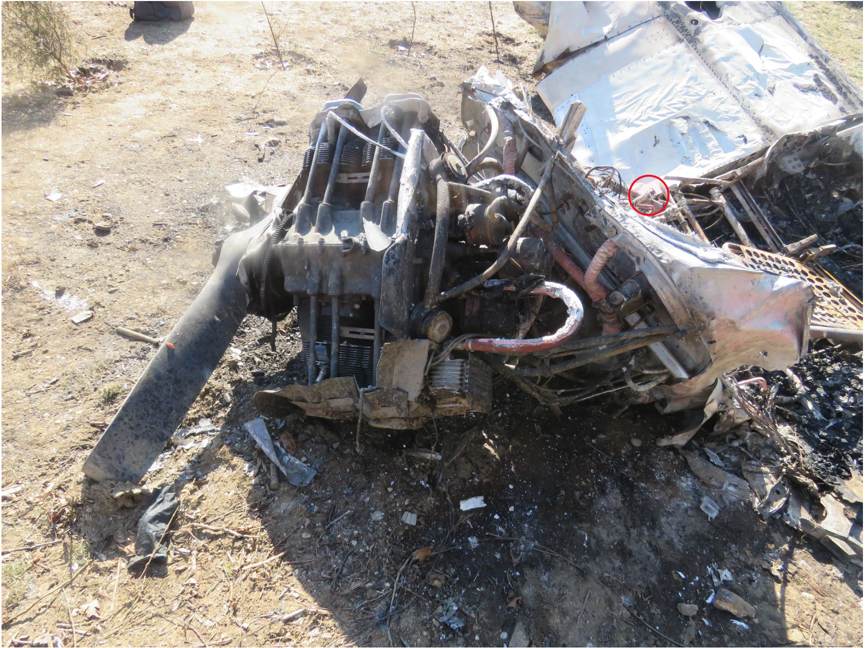
Photo 4 – View of Engine as Found (Lycoming)
