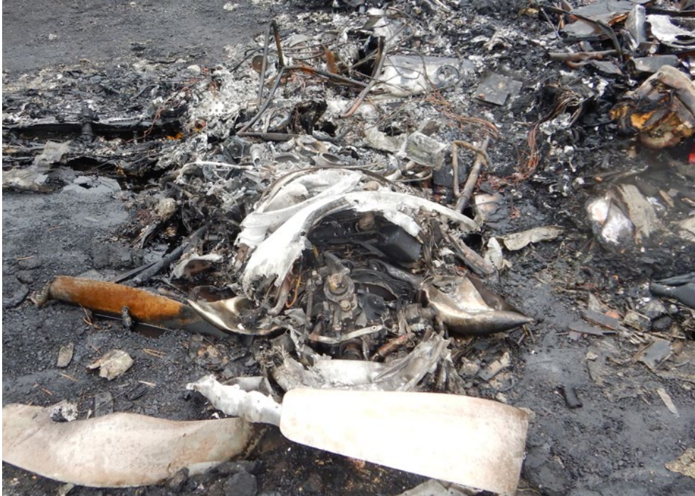
Figure 6 Right engine Assy embedded in pavement.
