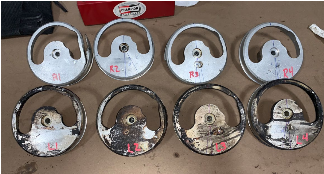
Figure 8 Propeller preload plates indicate blade angle at time of impact. Photo courtesy of Hartzell.
