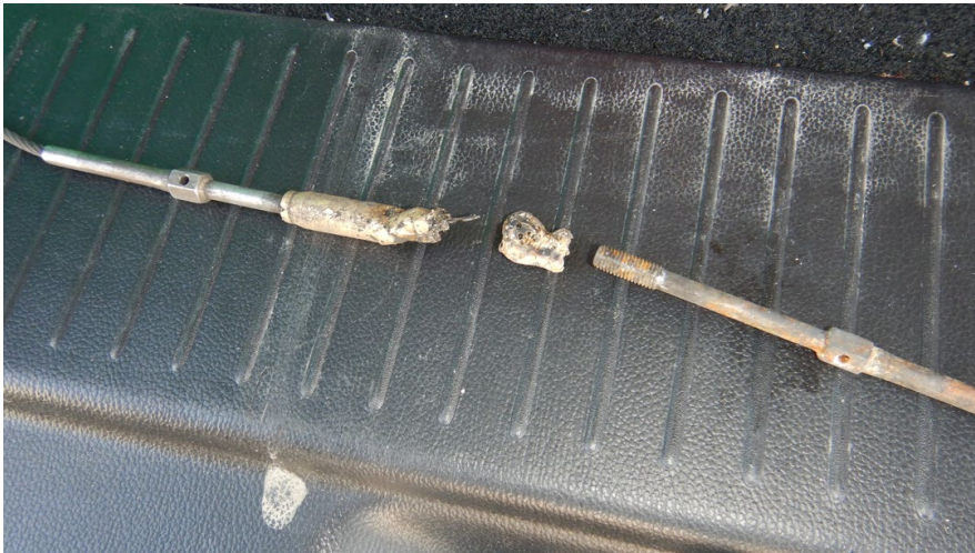
Figure 3 Elevator cable and turnbuckle. Visual exam revealed it was melted post impact.
