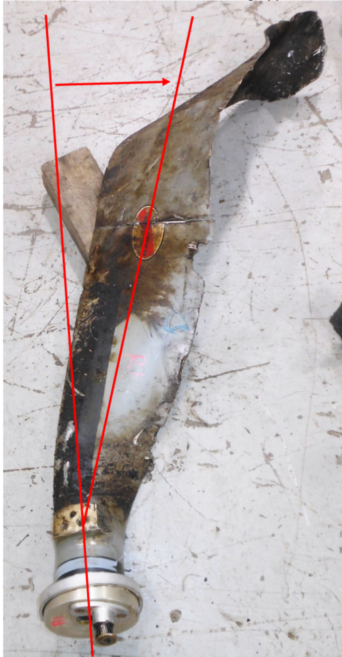
Photo #27 - Blade R1 remarkable bending opposite rotation
