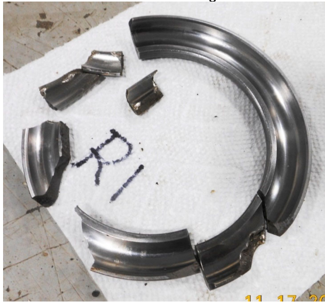
Photo #22 - Blade R1 bearing race fractures
