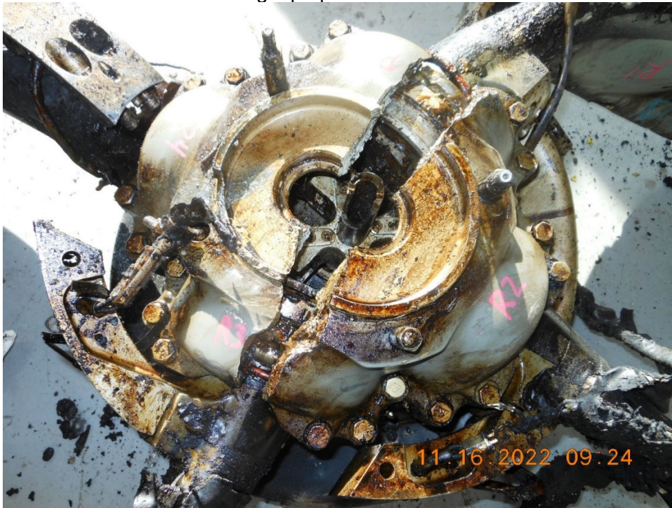
Photo #16 – Right propeller forward hub fracture
