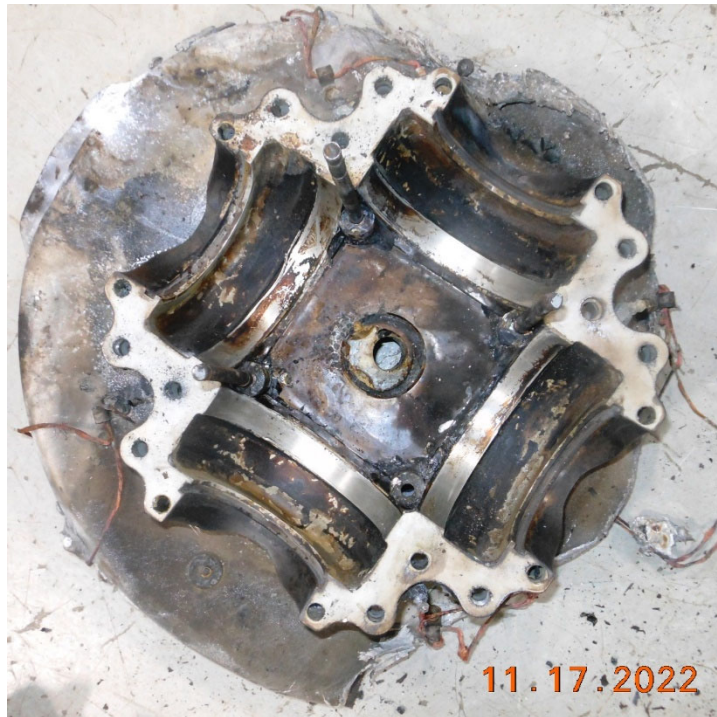
Photo #10 – Left aft hub half internal surface
