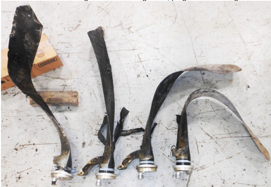
Photo #24 – Right blades trail edge view, progressive bending
