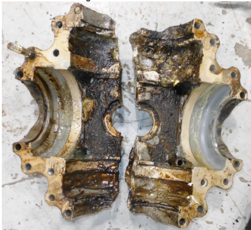
Photo #19 – Right forward hub half internal surface
