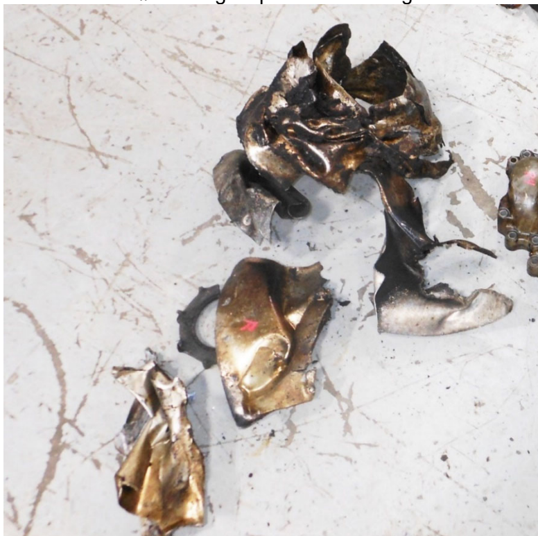
Photo #17 – Right spinner dome fragments
