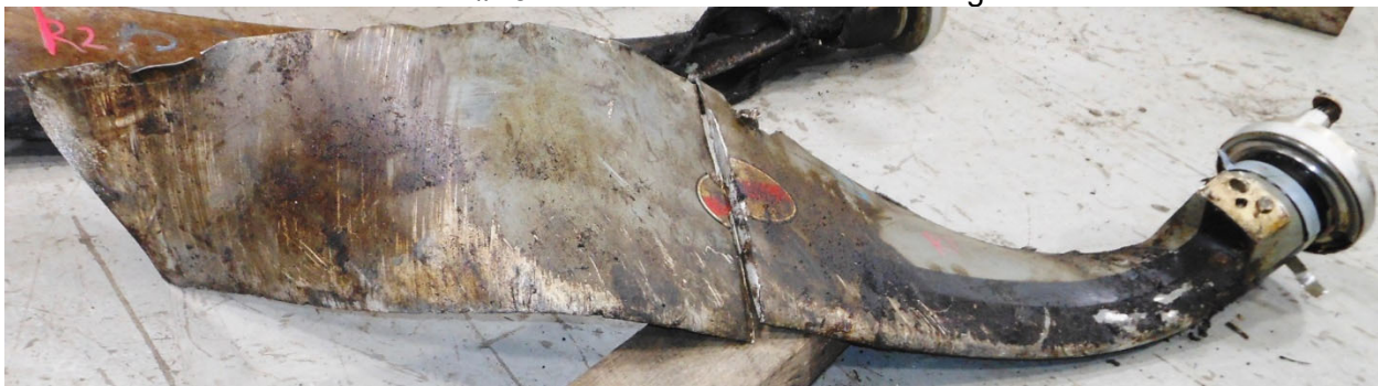
Photo #25 - Blade R1 camber side damage
