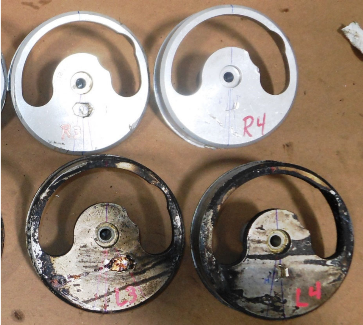
Photo #3 – Similarity of preload plates R3-L3 and R4-L4
