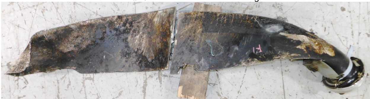
Photo #26 – Blade R1 face side damage
