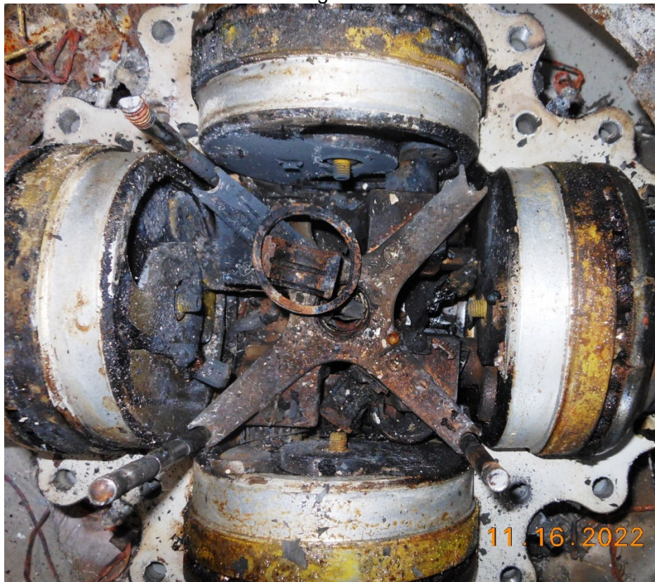
Photo #6 – Pitch change mechanisms condition
