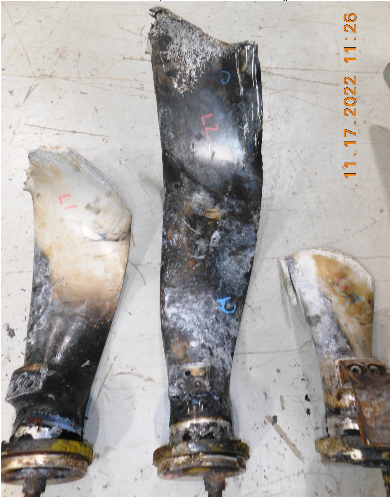
Photo #13 – L1, L2 and L3 relative heat damage
