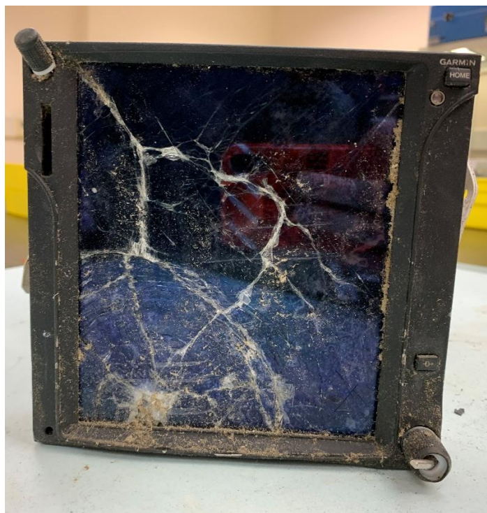
Figure 2. Photo of Garmin 750 showing impact damage.
