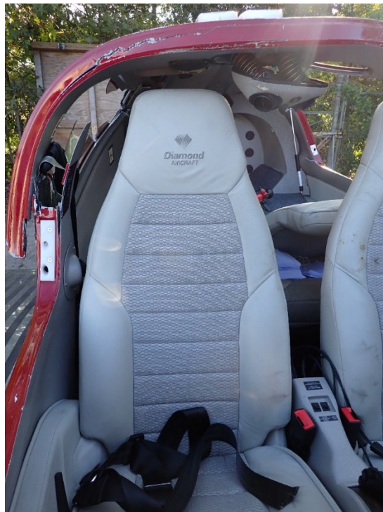
Figure 8. Right-hand pilot seat at salvage yard with cut upper torso webbing laying in the seat.
