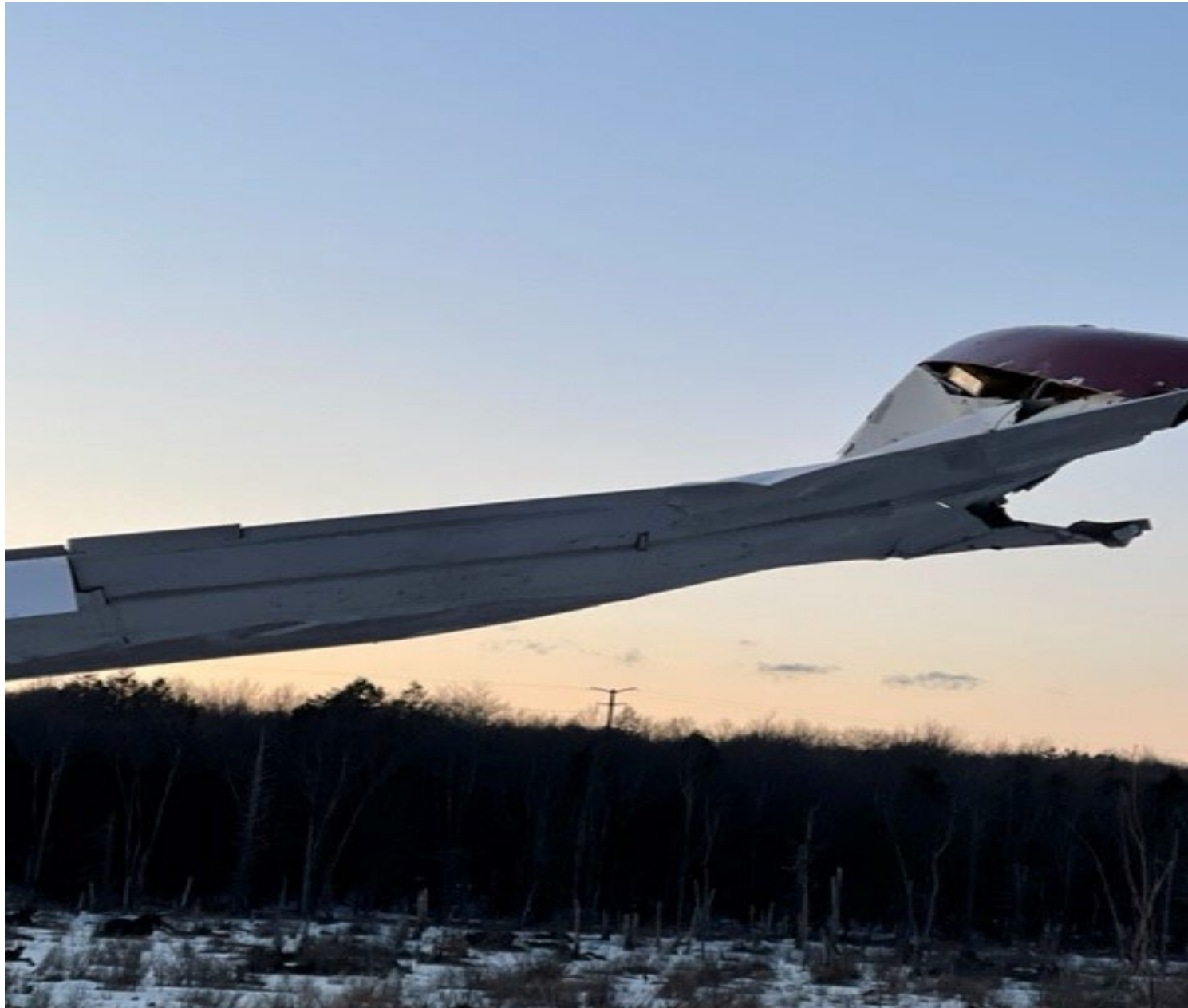
Photo 2 – View of Damage to Right Wing, Wingtip, and Aileron Hinge Mount (FAA)
