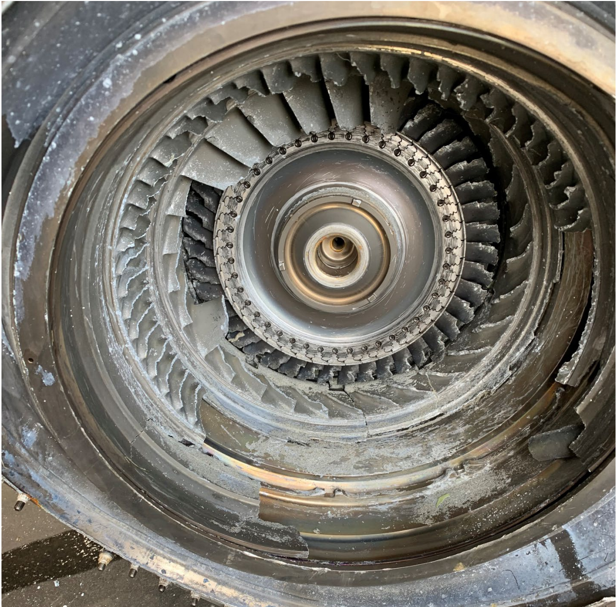
Figure 9. View of turbine vane airfoils bent the opposite direction of travel and rotational scoring throughout engine.
