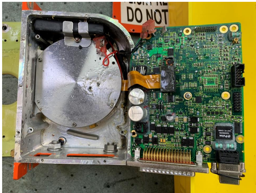
Figure 2. The internal condition of the LDR.
