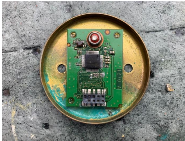
Figure 4. The internal memory module upon removal from the LDR.
