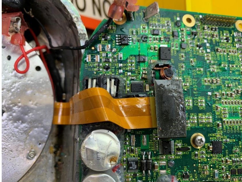
Figure 3. A close up of the memory module's ribbon cable.
