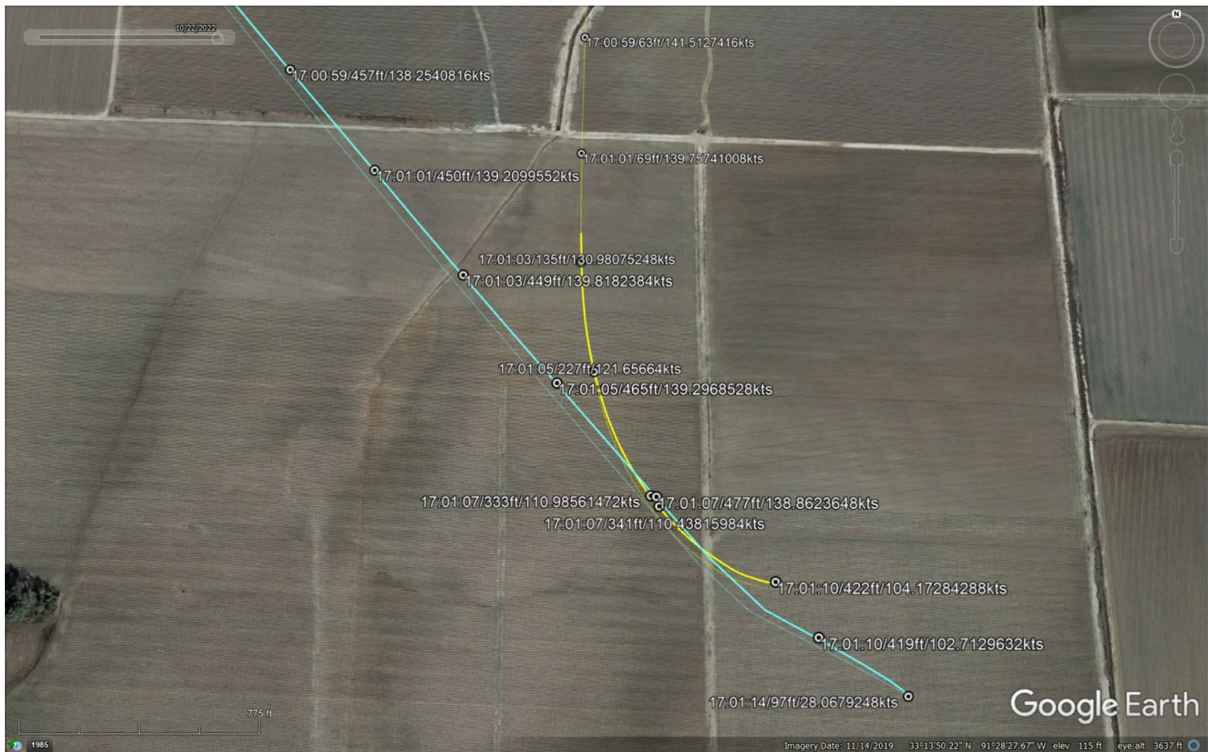
Figure 4. Google Earth overlay showing approximately the final 15 seconds of recorded data from the SATLOC G4 (N749LA, in yellow) and AgPilotX (N214RL, in cyan).
