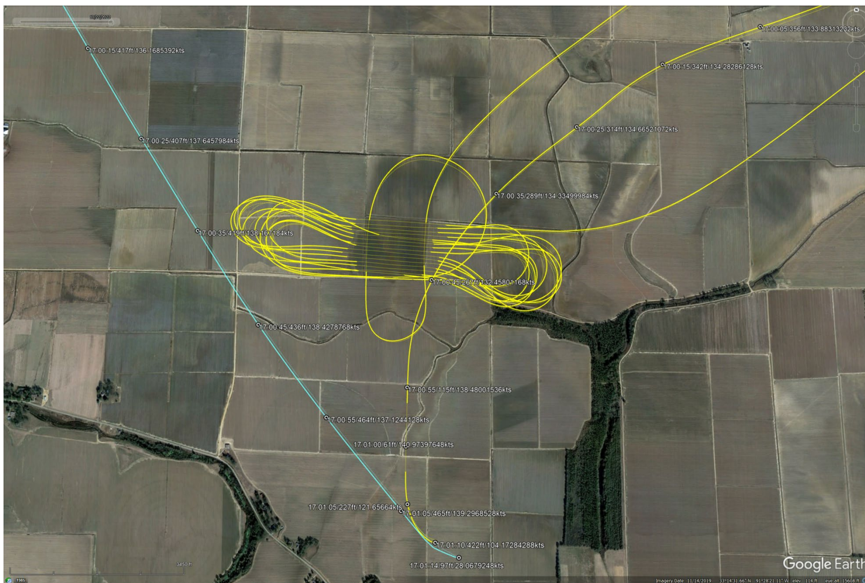
Figure 3. Google Earth overlay showing approximately the final minute of recorded data from the SATLOC G4 (N749LA, in yellow) and AgPilotX (N214RL, in cyan).
