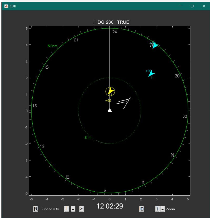
Figure 23c. Simulated CDTI display and view from the Cessna pilot seat at 12:02:29 (22 seconds before the collision). The Piper is located in the yellow circle. AIRCRAFT PERFORMANCE & COCKPIT VISIBILITY STUDY
