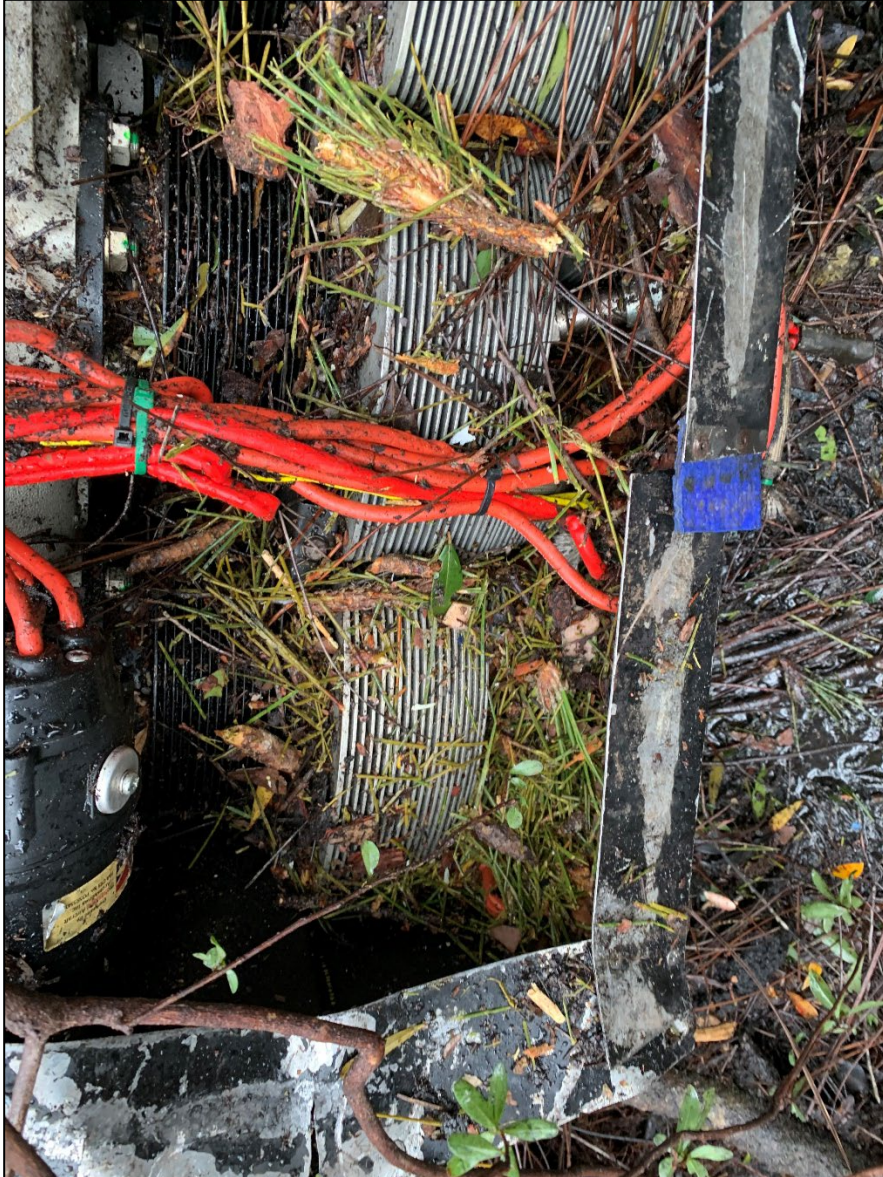
Photo 8: View of small chopped up pine tree debris located spread across the top and rear of the engine.
