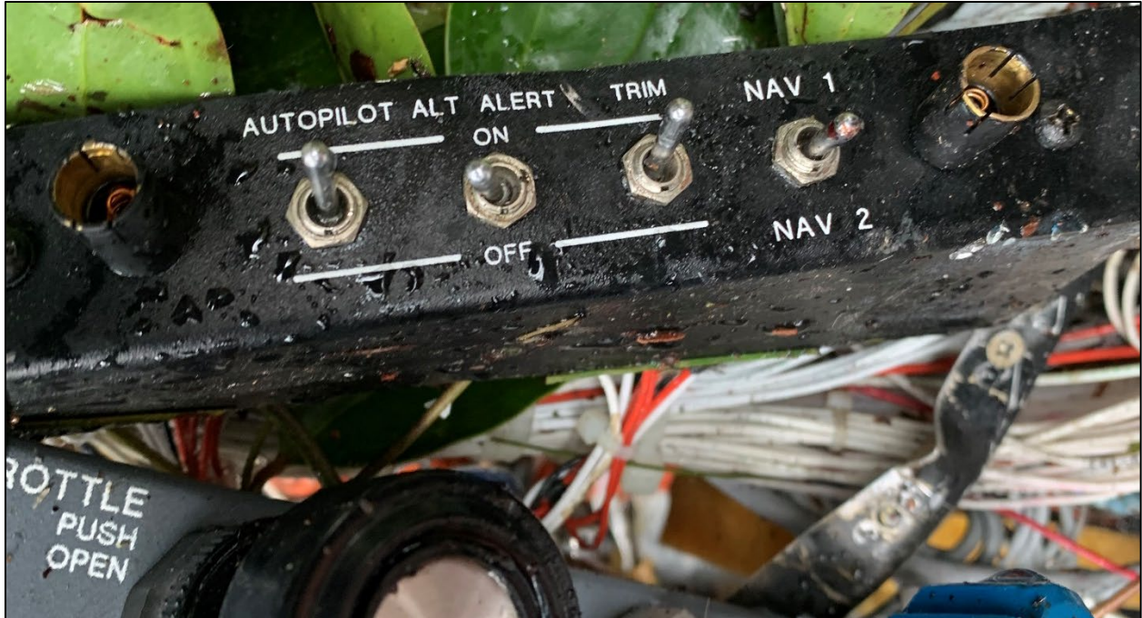
Photo 6: View of the autopilot, altitude alerter, and elevator trim ON/ OFF mode control panel
