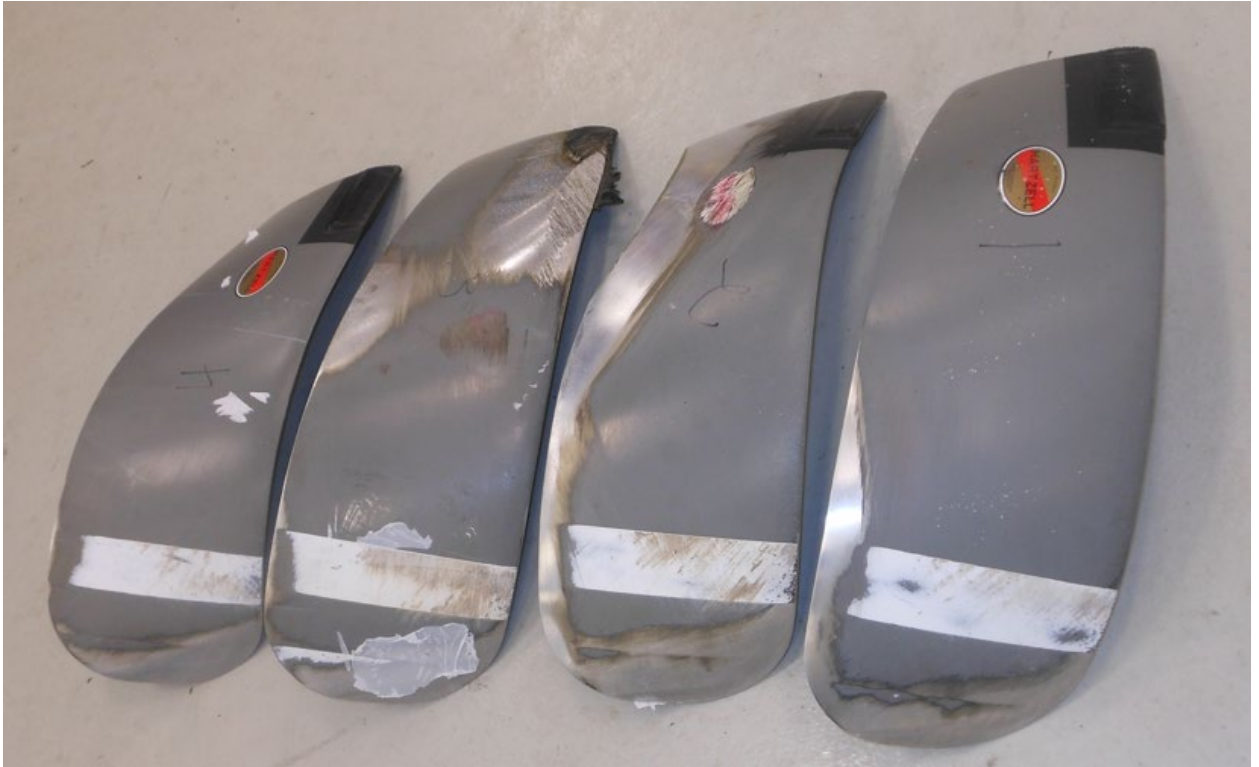
Photo #2 - Blade damage
