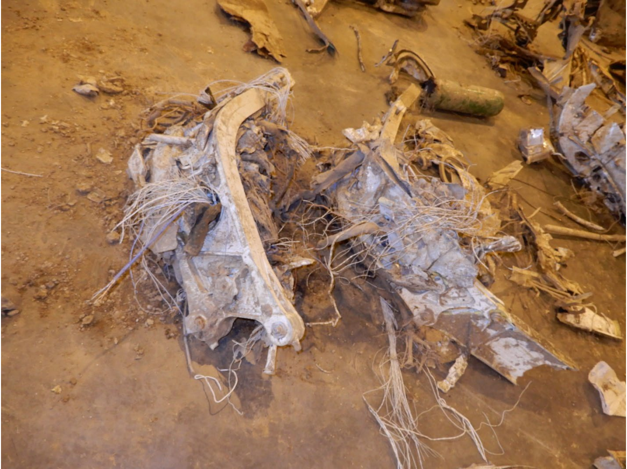
Figure 2. View of forward and aft sections of center wing spar.
