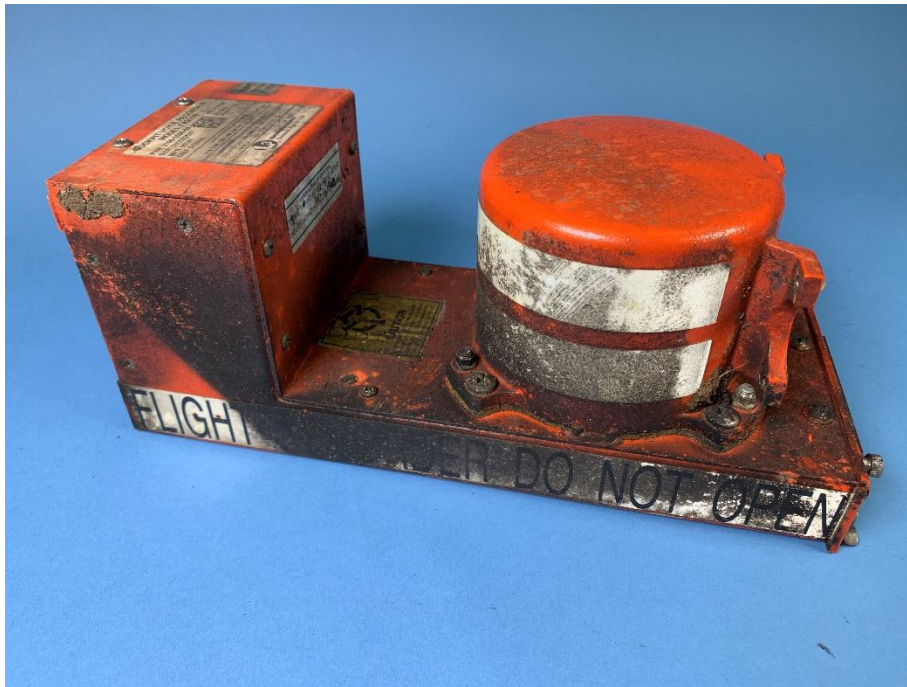
Figure 1. The arrival condition of the CVR from N560AR.
