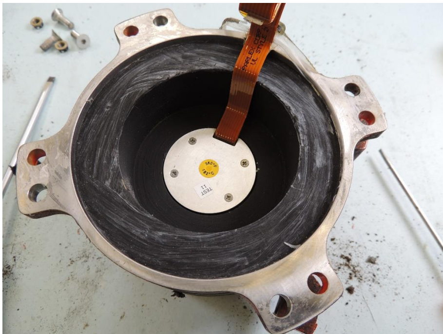
Figure 2. The condition of the CSMU and associated NVM chip stack.
