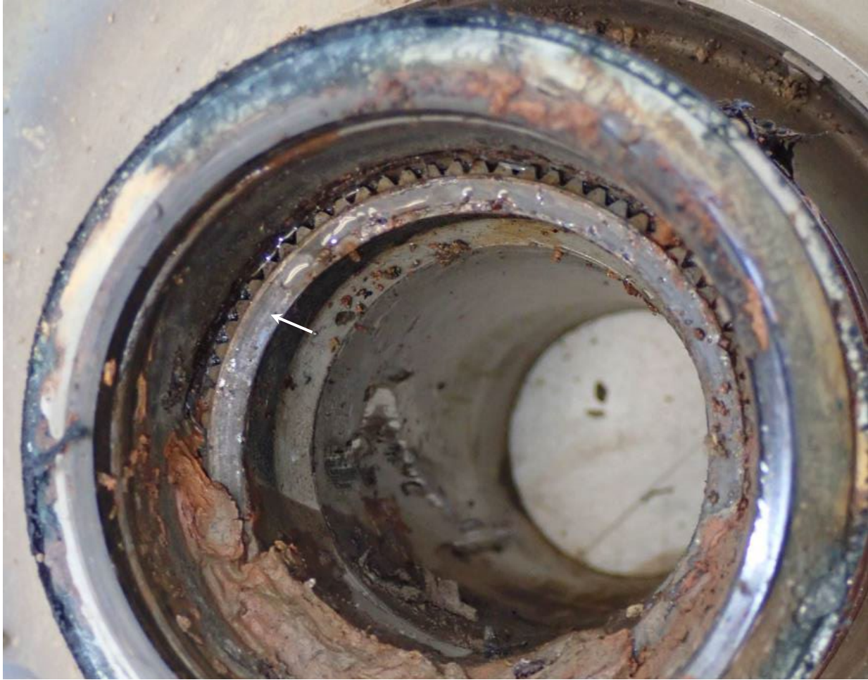
Figure 15. Post-separation rotational scoring to the high turbine shaft fracture surface
