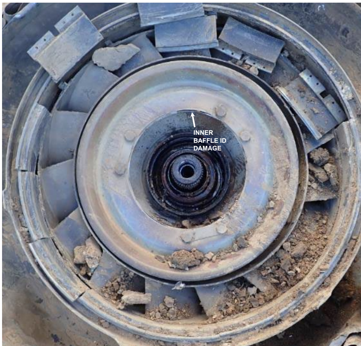
Figure 16. Downstream view of the high turbine stator assembly showing circumferential scoring at inner baffle ID
