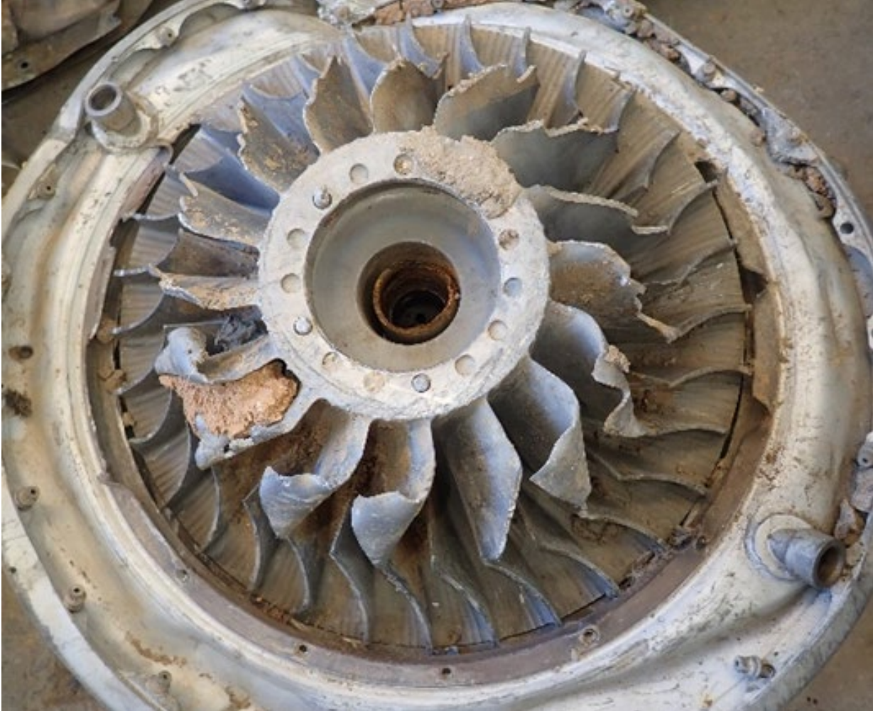
Figure 13. Right engine front view showing impeller damage
