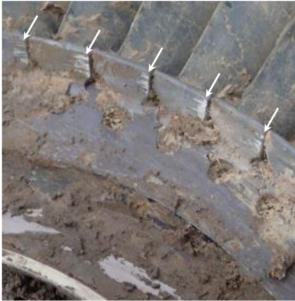
Figure 21. T3 blade under platform rub
