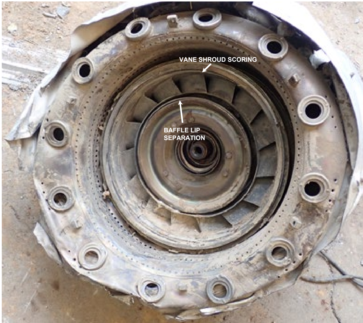
Figure 3. Downstream view of the high turbine stator, showing 360° rub at the shroud and the baffle lip
