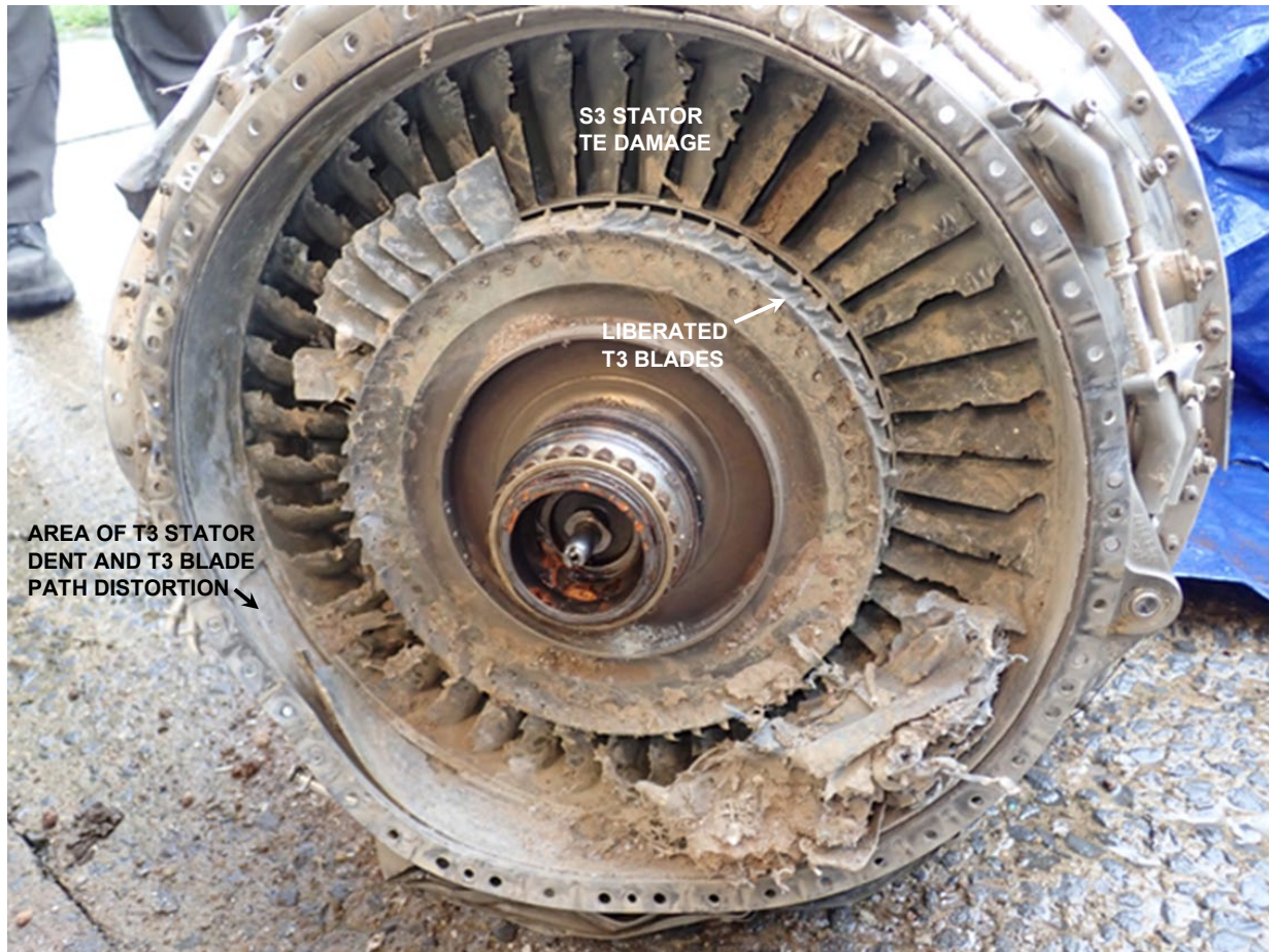
Figure 11. View of the aft end of the low turbine rotor showing deformed T3 blade path, liberated T3 blades and T3 stator trailing edge damage
