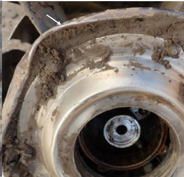
Figure 22. Local circumferential scoring to turbine exhaust duct inner shroud
