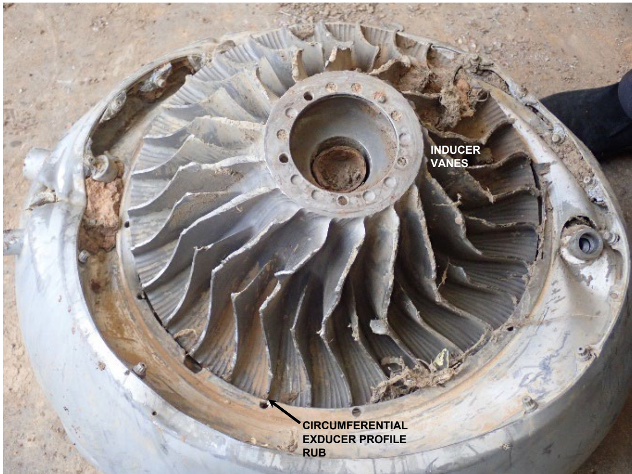
Figure 2. Front view of engine S/N 77407 showing impeller damage
