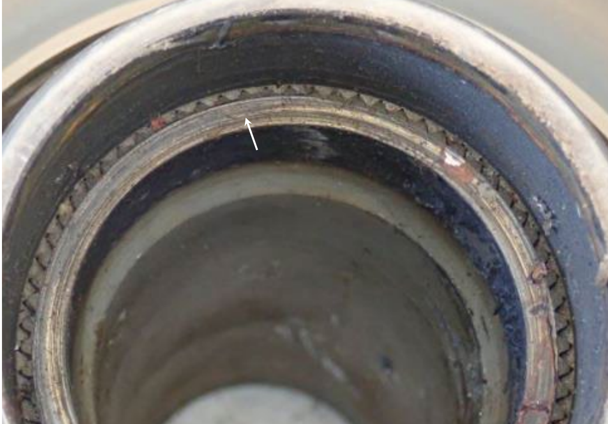
Figure 8. Rotational scoring damage marring the high turbine shaft fracture surface
