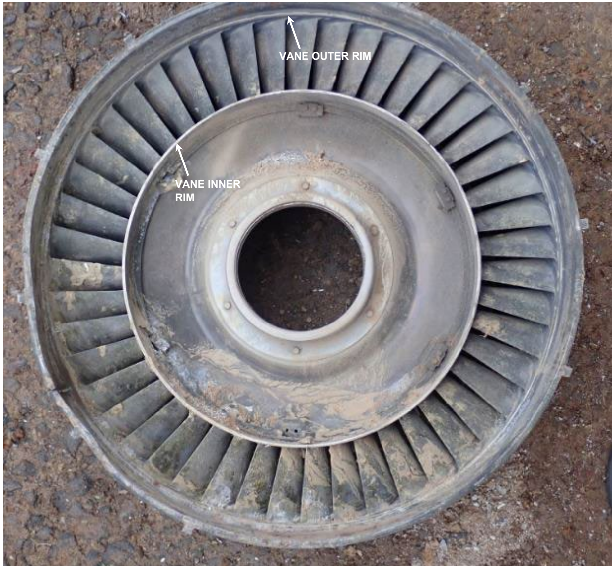
Figure 9. T2 stator downstream side showing 360° scoring along the vane inner and outer rims
