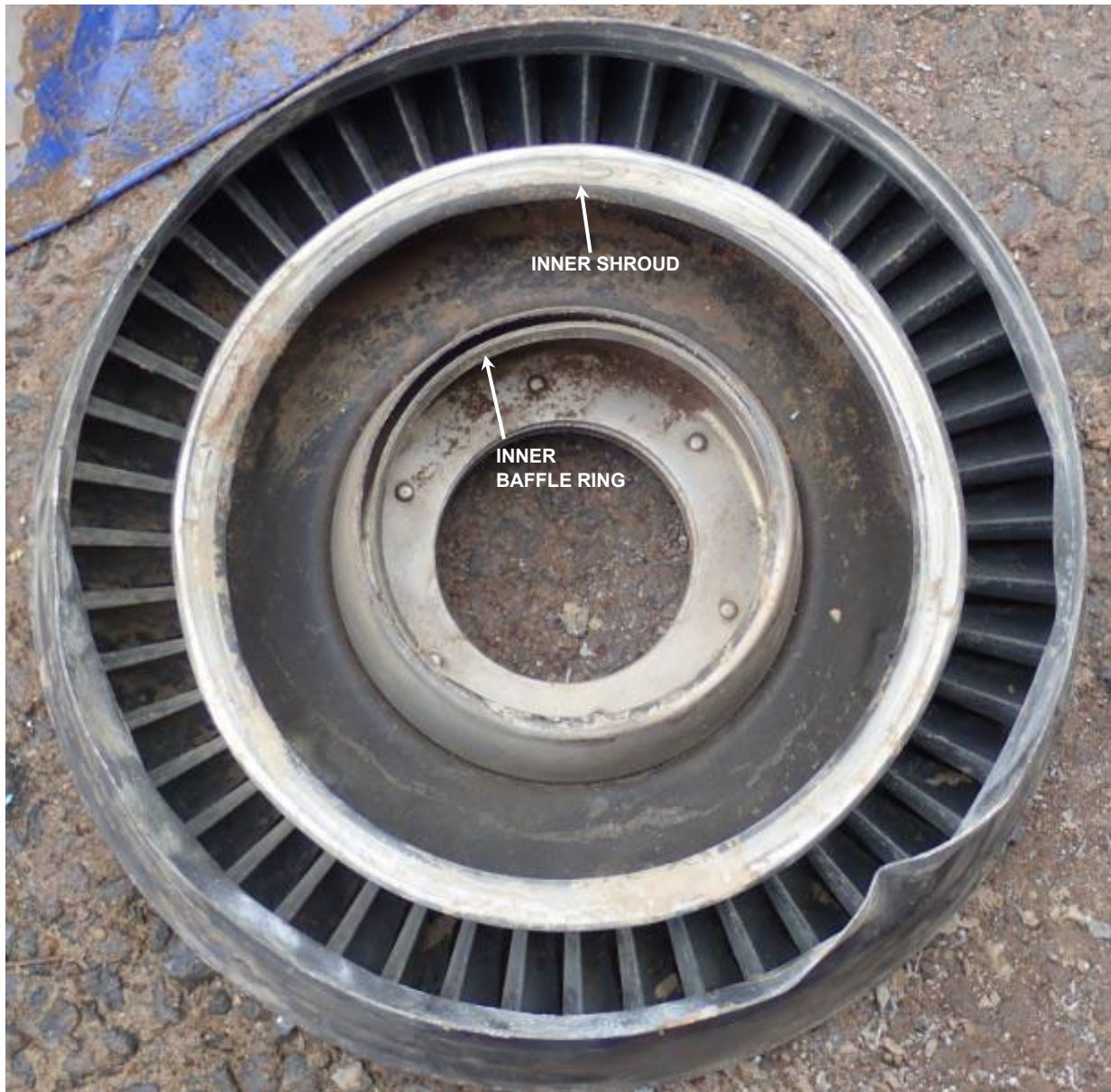
Figure 7. T2 stator upstream side showing 360° scoring damage along vane inner shroud and inner baffle ring
