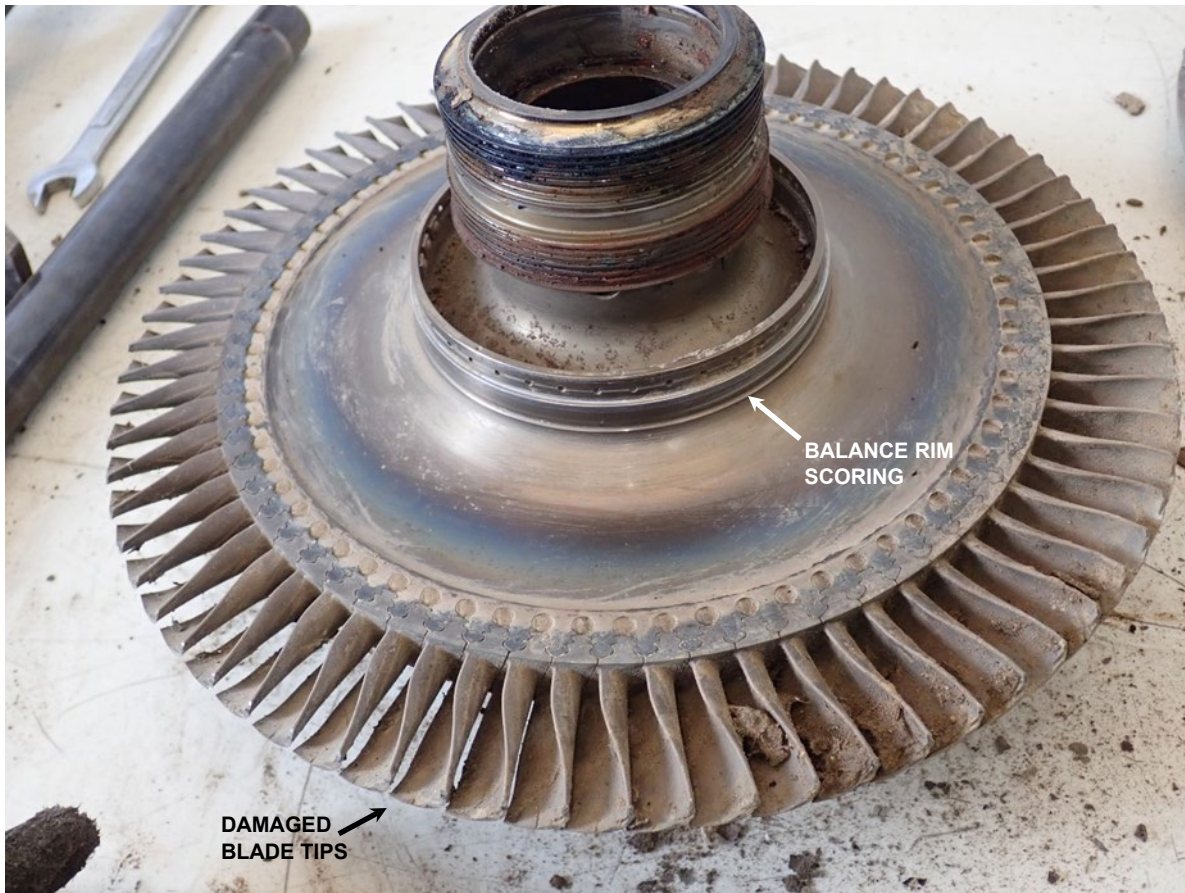
Figure 17. Upstream face of high turbine showing 360° scoring damage at the balance rim
