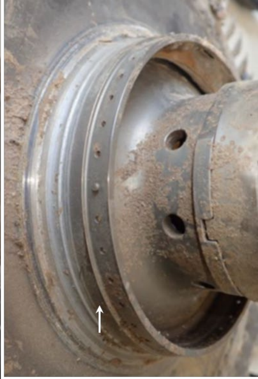
Figure 6. 360° scoring at high turbine balance flange
