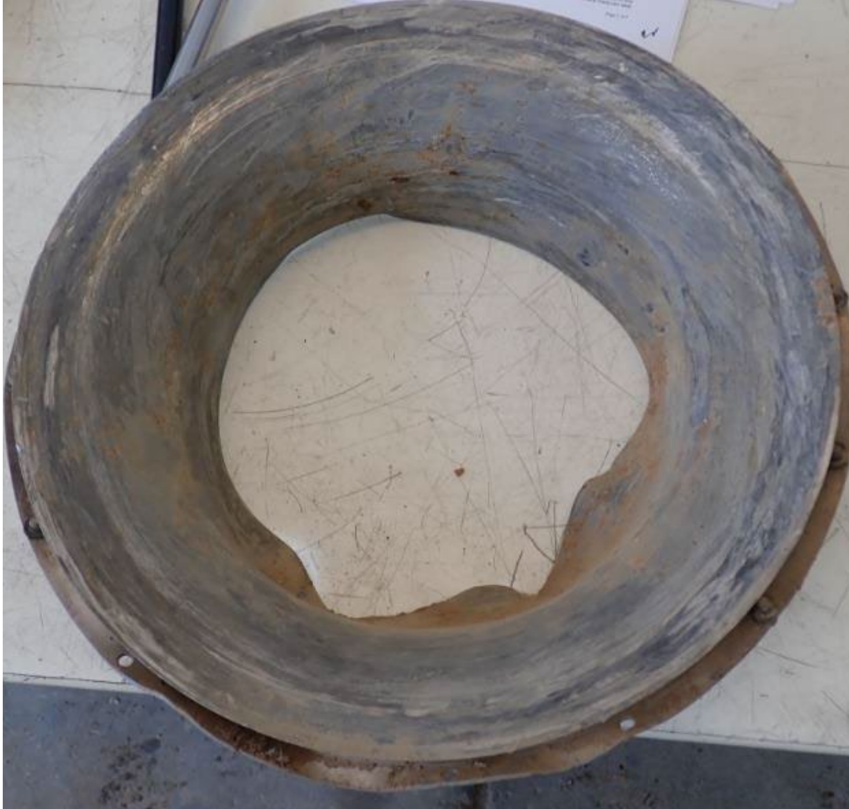
Figure 14. Impeller housing/shroud showing rotational scoring
