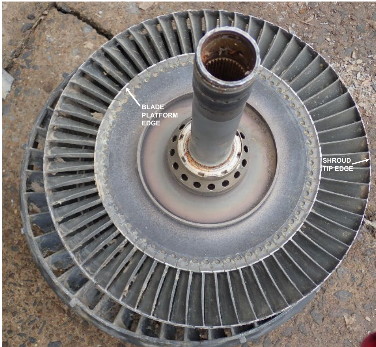
Figure 10. T2 showing circumferential rub along the blade platform and shroud tip edge
