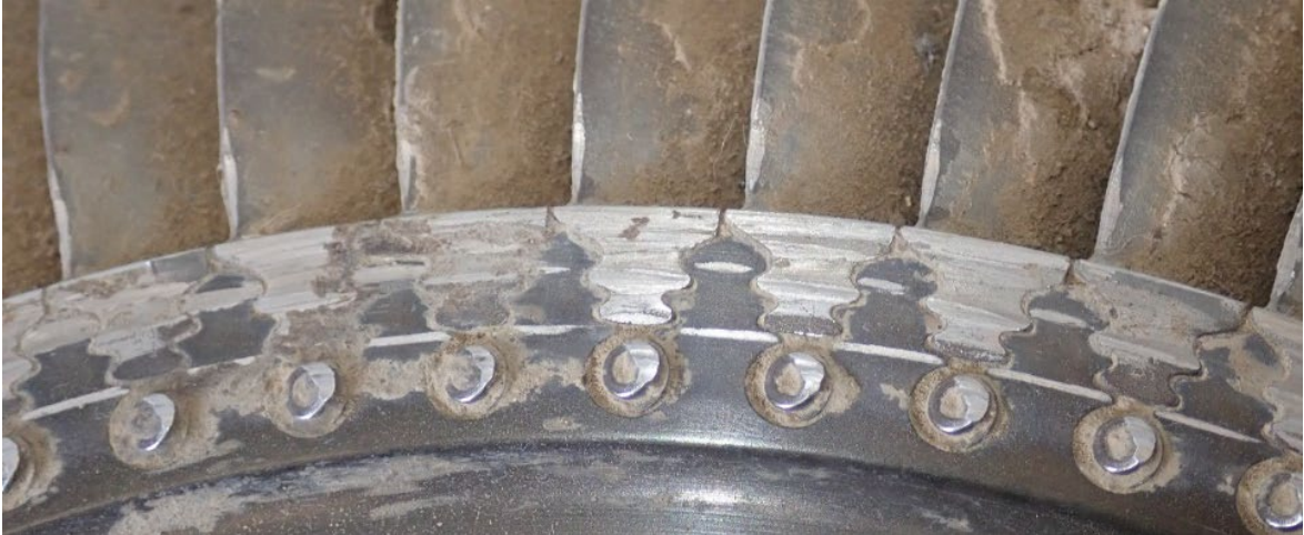
Figure 19. Detail of circumferential scoring along fir tree/blade area on high turbine downstream face
