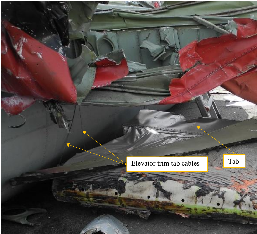
Figure 20 Left elevator trim tab cables
