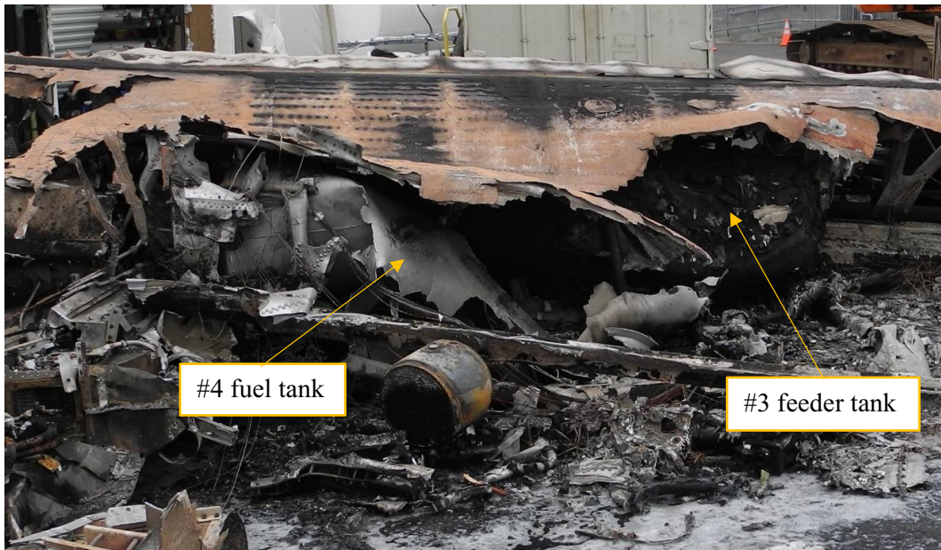
Figure 32 Right wing fuel tanks
