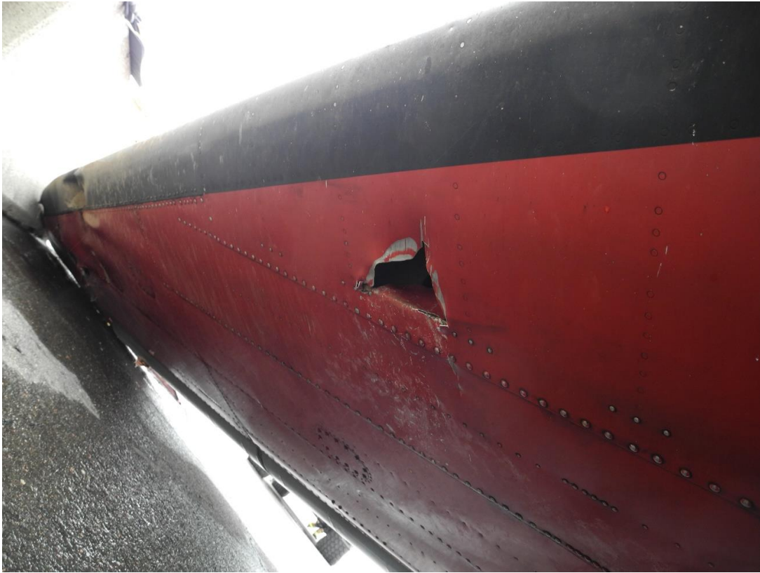
Figure 16 Right horizontal stabilizer impact damage
