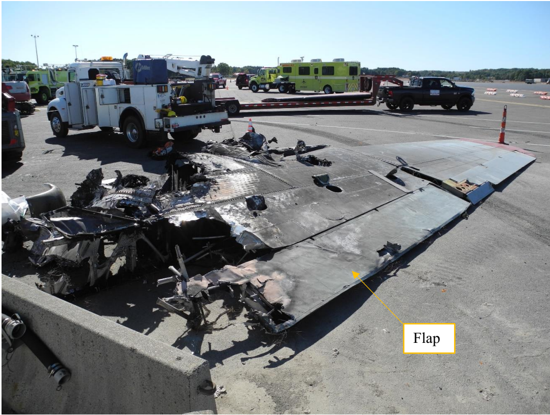
Figure 4 Left wing upside-down to show flap
