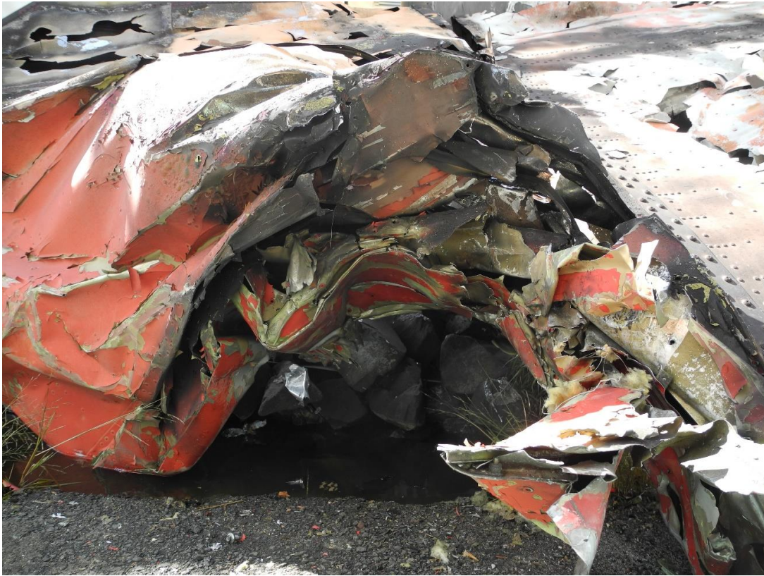
Figure 9 Right wing tip impact damage
