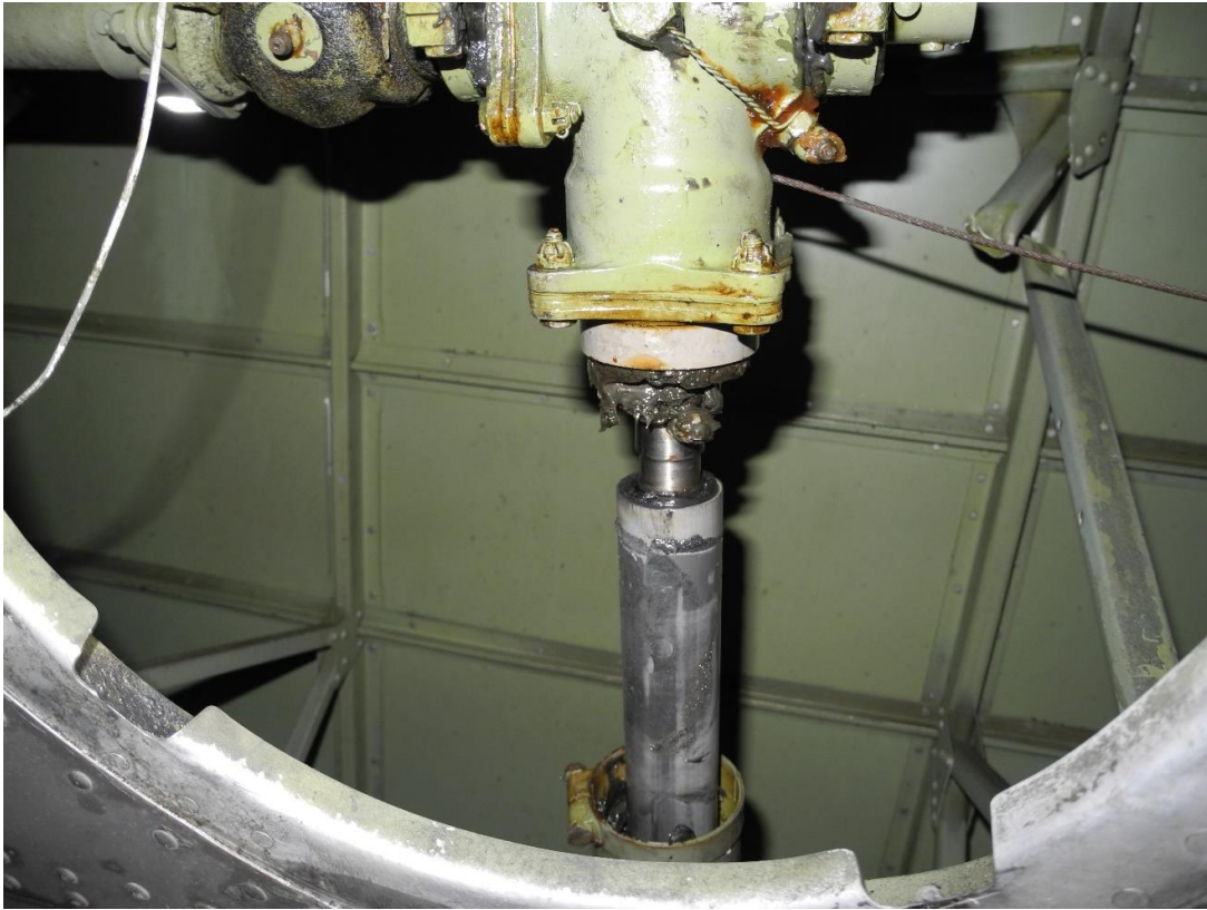
Figure 5 Flap drive and jackscrew
