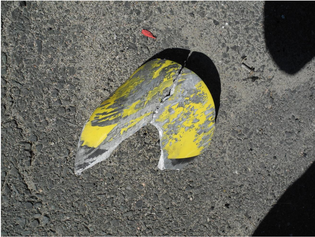
Figure 47 Fractured #3 Engine propeller tip (two pieces)
