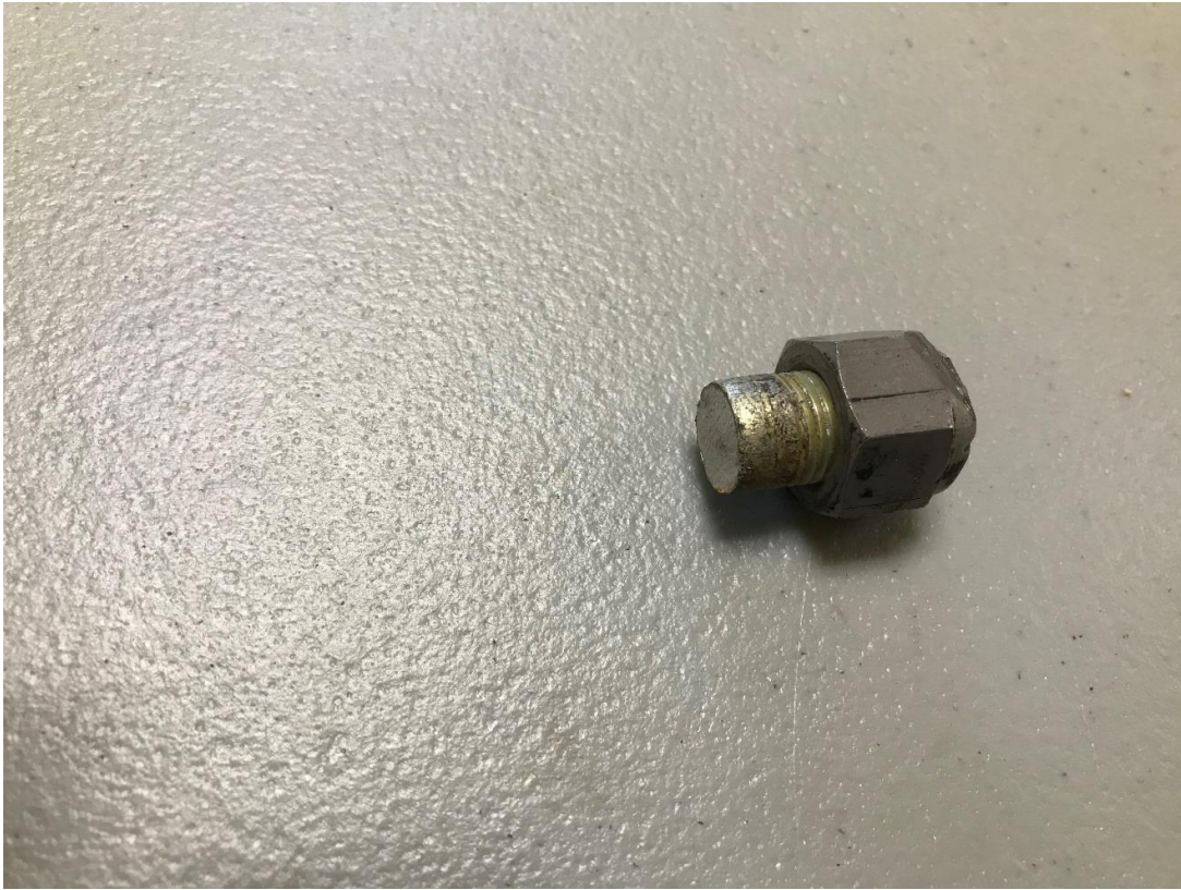
Figure 22 Bottom half of fractured shear bolt
