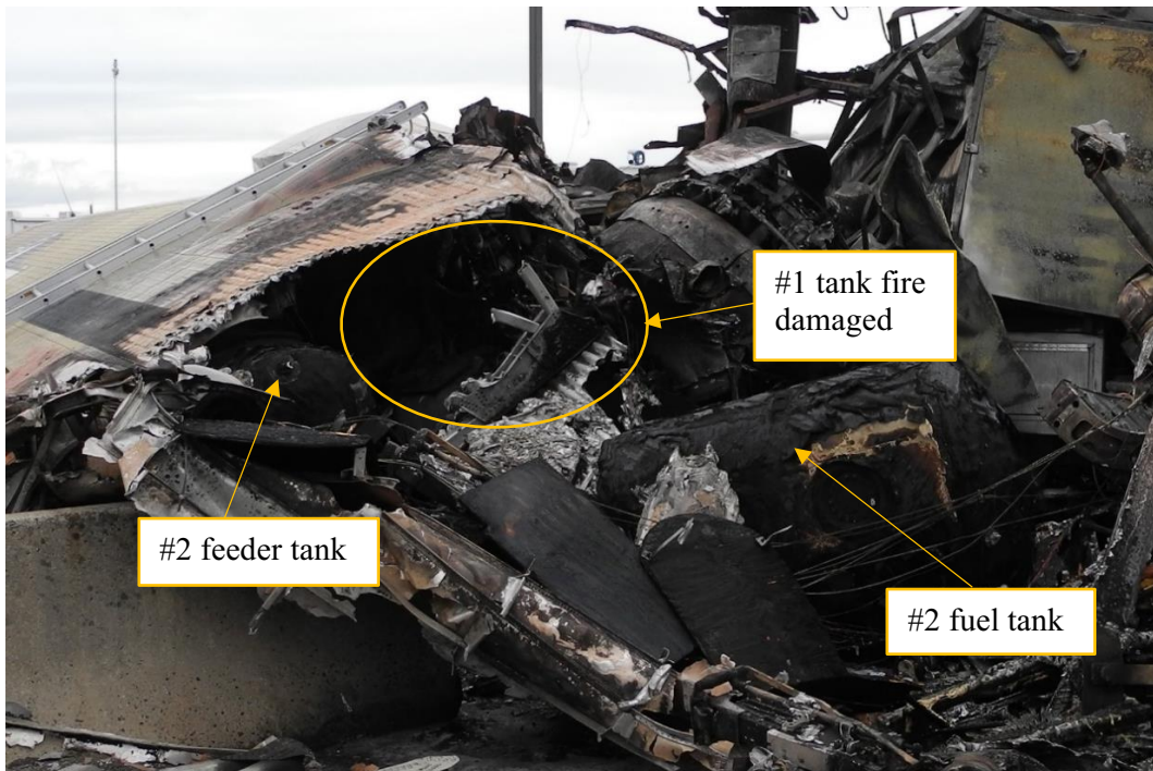
Figure 31 Left wing fuel tanks
